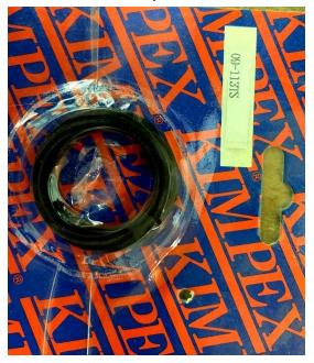
Unfortunately the new seal had a 42mm outside diameter, so I needed to make a spacer ring.
