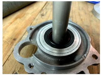
Here's the fun part, due to the way the motor is built, a leak at this seal will allow coolant into the motor, where I think it could pass through the power conductor passage into the inverter housing. I decided I'd rather dump the coolant overboard if it were to leak again. (which I anticipate it will, since I don't think my replacement seal is as good as the original)
