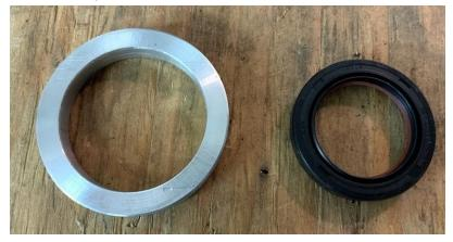
I used Permatex sleeve retainer to hold and seal the spacer ring into the housing, and pressed everything together:
