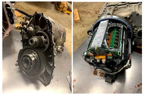
When reassembling the gearbox, make sure the parking pawl is disengaged. (picture shows it engaged) You can manually disengage it with a  $\frac{1}{4}$ " socket. If the case halves don't go together easily, it's probably the parking pawl.
