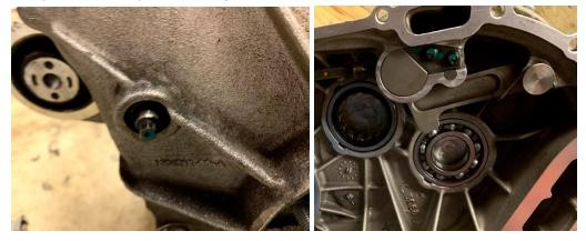
Once reassembled, you will want to make sure the small coolant hole is clear of sealant. I used a pick to reach into the passage.
