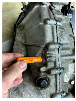
Replacing the axle seals was very easy. Just pop the old ones out with a pry bar, and hammer the new ones in with a large socket. Just make sure not to drive the new seals in too far, there are no stops inside the gearbox. The replacement seals are purchasable directly from Toyota. There are a few other external parts of the drive unit available from Toyota as well. The seal part number is 17292-0Z010.
