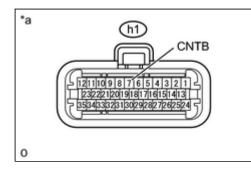
(a) Disconnect connector h1 from the electric vehicle battery.
