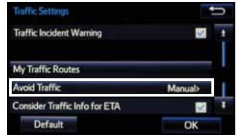
**step 2** Select the **Avoid Traffic** option to switch from Manual to Automatic and press **OK**. The system will automatically select another route when moderate or heavy traffic is detected during route guidance.
