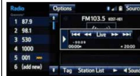
The Audio App features a pause function that will record up to 20 minutes of live radio for playback later. The **Tag** feature will record a song from live radio for purchase from a paired mobile device later.
