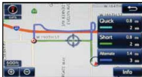
One of three routes may be chosen for the trip: **Quick**- is the easiest route, usually the fastest **Short**- is the most direct based upon driven mileage **Alternate**- is the second fastest route
