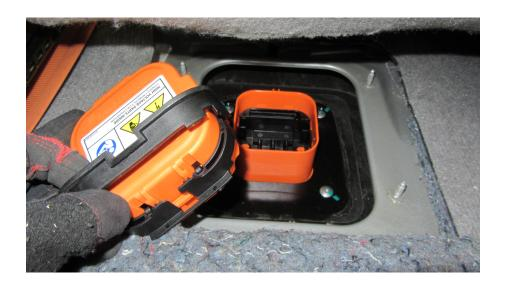
10) Drill / ream the high voltage disconnect cover bolt holes with a 1/4" drill bit for easier removal and installation of cover later.
