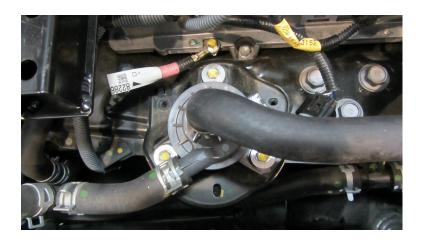
18) Remove bolt from cabin heater hose support as depicted (use 10mm socket with long 1/4" square drive extension)
