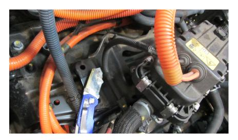
17) Remove two bolts (10mm socket and long 1/4" square drive extension) from cabin heater water pump, after removing wire / cable connector and removing cooling hose clip / attachment.
