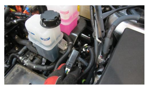
33) Plug correct wiring harness connector into onboard charger, routing the plug as depicted. If the cable isn't routed correctly, it may rattle against the vehicle chassis
