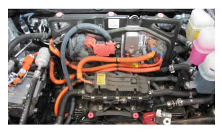
15) Remove four 10mm flange nuts from cabin heater mount and one 10mm flange nut from the cabin heater ground wire.
