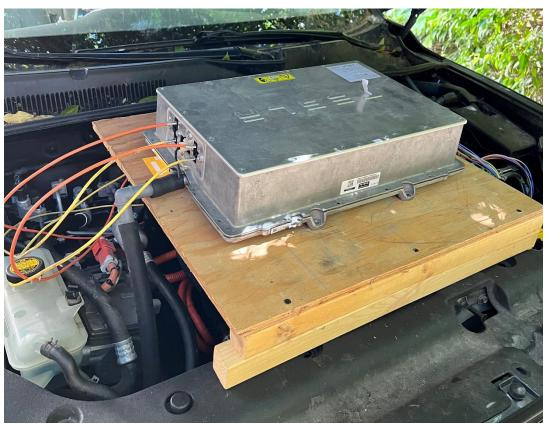
First, we mounted the replacement charger on the test bed and made all of the connections to the rest of the power train. As with the prior time, the car would not go into "READY" mode and the charger did not work. We disconnected and reconnected it a few times after checking a few things.
