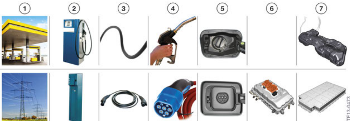
Components for refueling the vehicle and charging the high-voltage battery
