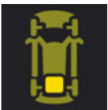
Check Control symbol for power reduction due to high temperature of electric motor components
