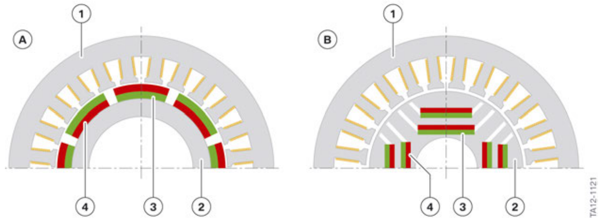
Principal structure of the synchronous machine
