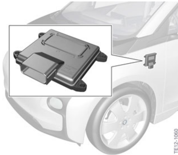
Installation location of the EDME
