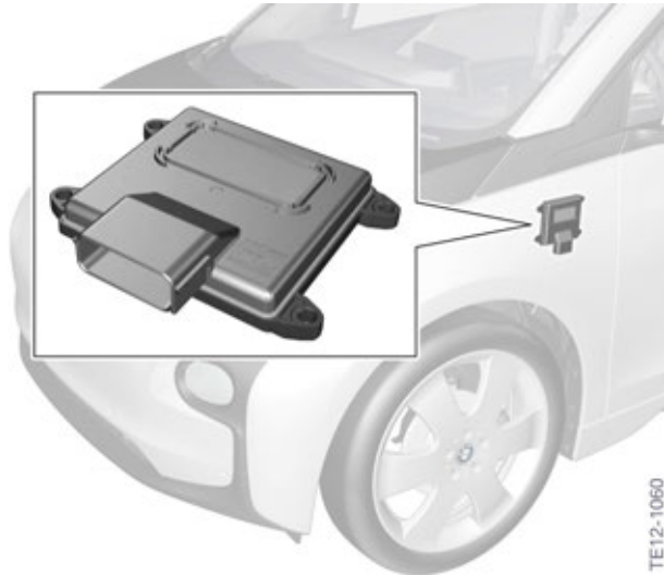
Installation location of the EDME
