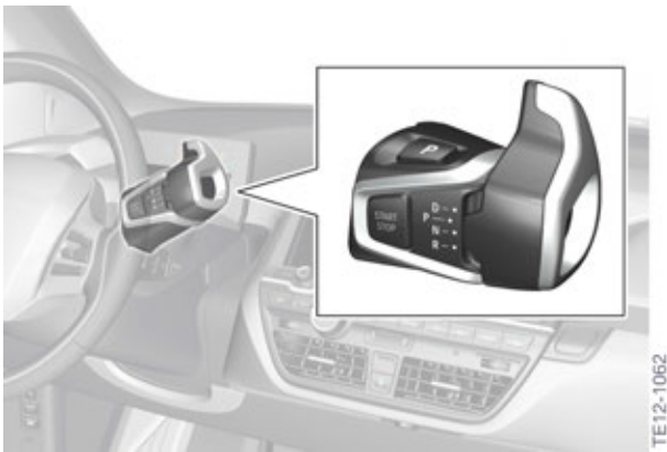
Gear selector switch I01
