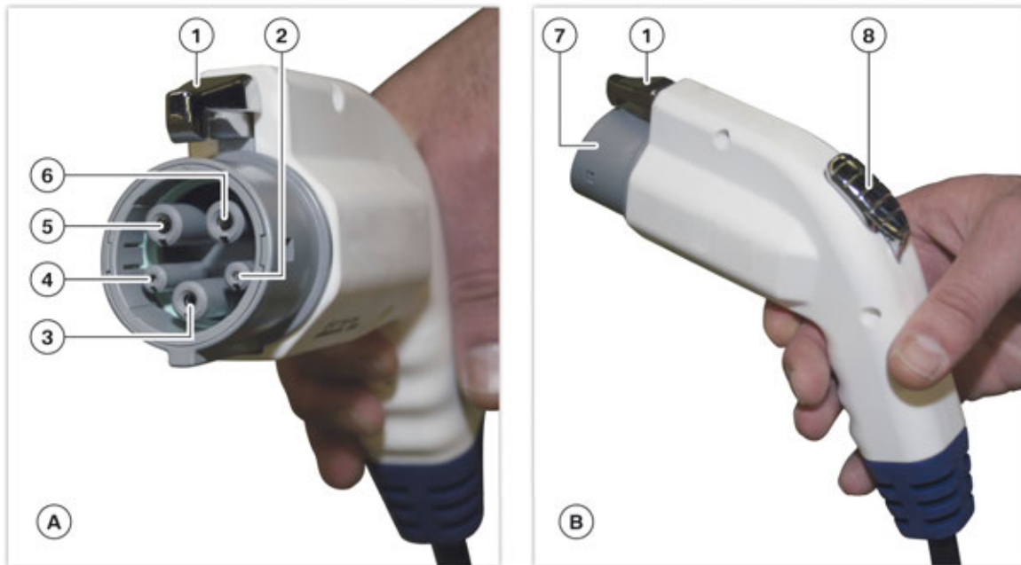
Connector of the charging cable for the connection to the vehicle (standardized i.a.w. IEC 62196-2: Type 1)
