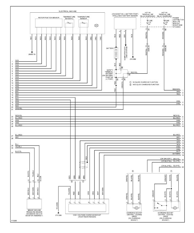
Fig. 42: Electric, Engine Performance Circuit (4 of 7)
