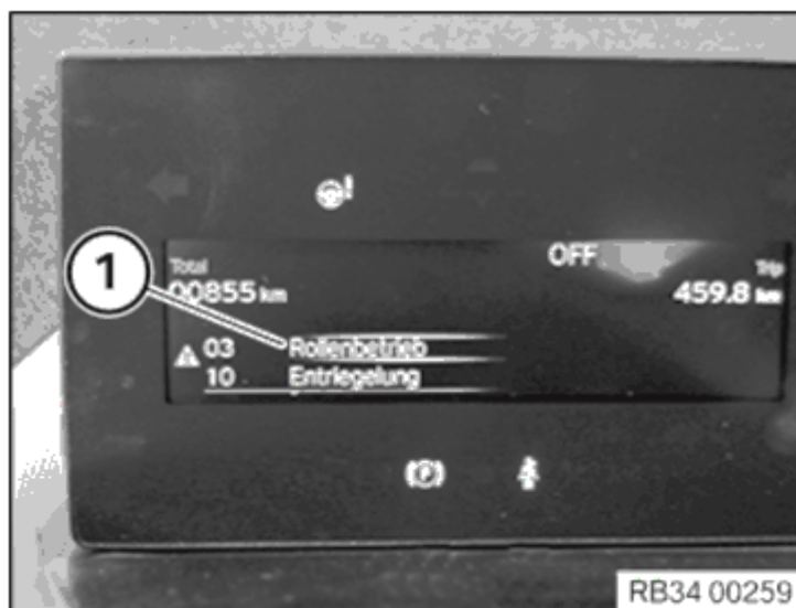
Fig. 9: Screen Display - 03 Roller Operation Menu Item Courtesy of BMW OF NORTH AMERICA, INC.
