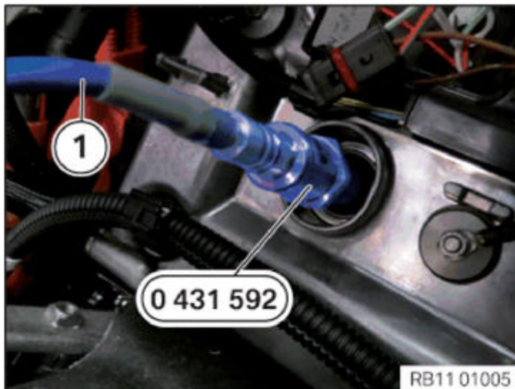
Fig. 5: Connecting Diagnostic Cable With Special Tool (0 431 592). Courtesy of BMW OF NORTH AMERICA, INC.
