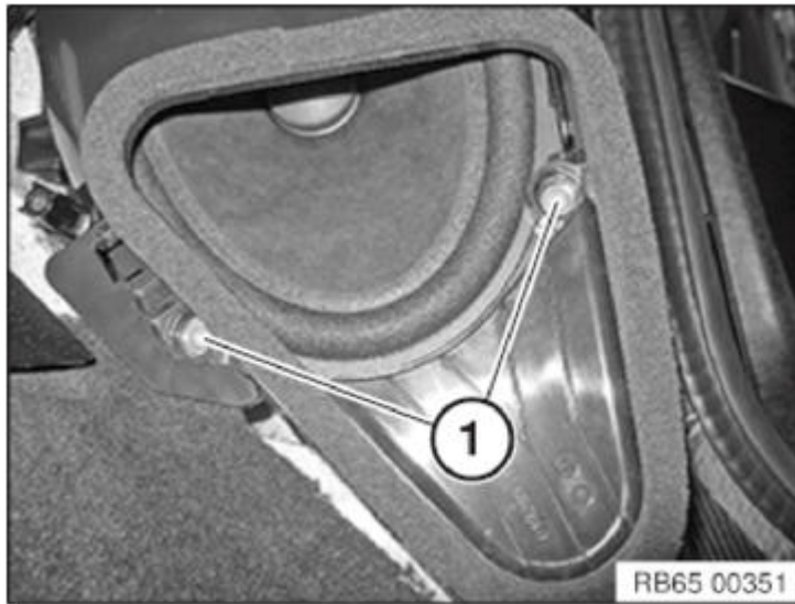
Fig. 11: Identifying Right Bass Speaker Screws Courtesy of BMW OF NORTH AMERICA, INC.
