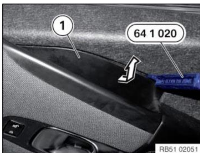
Fig. 301: Removing Cover Using Special Tool (64 1 020)
