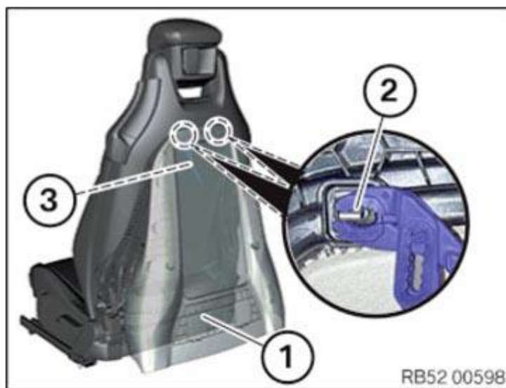
Fig. 12: Pressing Both Hooks At Clamps With Pliers Courtesy of BMW OF NORTH AMERICA, INC.
