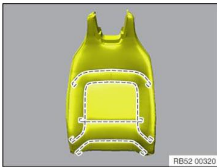
Fig. 56: Identifying Trim Wires Area
