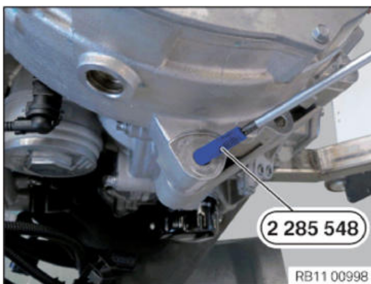
Fig. 28: Screwing Special Tool (2 285 548) M10 Into Torsion Spline Shaft Bolting Point Courtesy of BMW OF NORTH AMERICA, INC.
