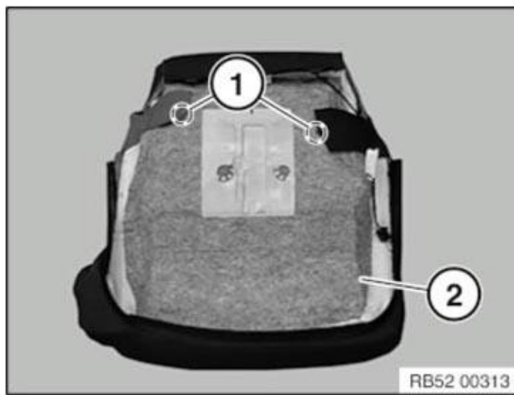
Fig. 61: Identifying Seat Cover And Clamps Courtesy of BMW OF NORTH AMERICA, INC.
