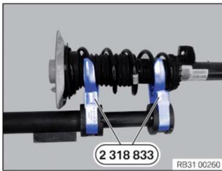
Fig. 71: Accommodating Coil Spring Using Special Tools (2 318 833) Courtesy of BMW OF NORTH AMERICA, INC.
