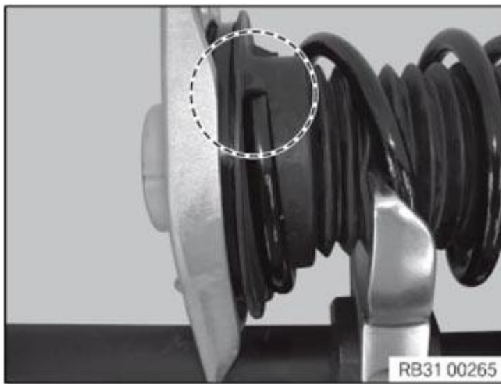
Fig. 89: Checking Top Spring Pad Position Courtesy of BMW OF NORTH AMERICA, INC.
