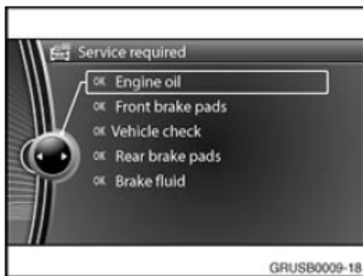
Fig. 5: Central Information Display - Service Required Screen Courtesy of BMW OF NORTH AMERICA, INC.
