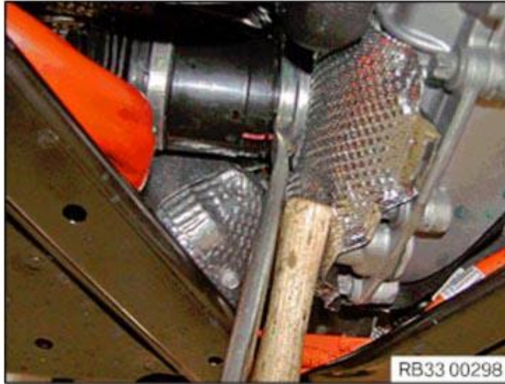
Fig. 17: Supporting Output Shaft Mounting Lever Using Wood Piece Courtesy of BMW OF NORTH AMERICA, INC.
