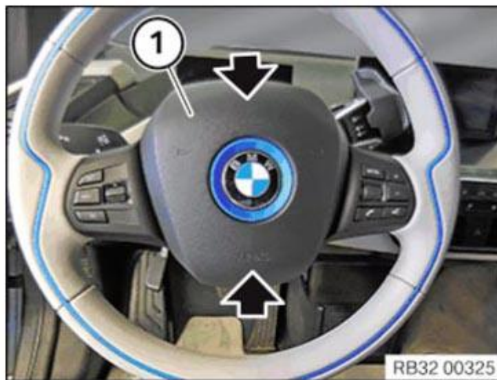
Fig. 63: Identifying Airbag Unit Pressing Direction Courtesy of BMW OF NORTH AMERICA, INC.
