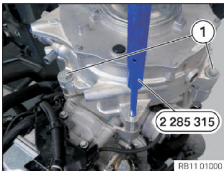
Fig. 41: Inserting Torsion Splined Shaft Screws Courtesy of BMW OF NORTH AMERICA, INC.
