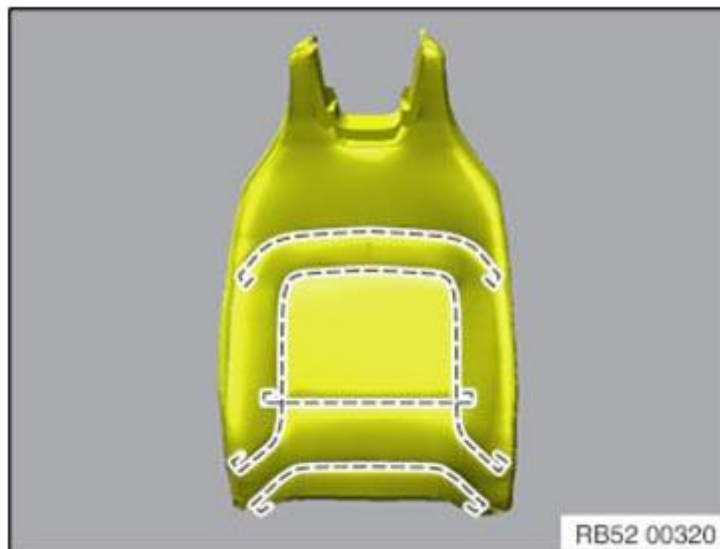
Fig. 49: Identifying Trim Wires Area
