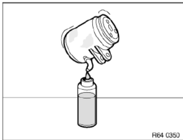
Fig. 173: Draining Refrigerant Oil Into Container Courtesy of BMW OF NORTH AMERICA, INC.
