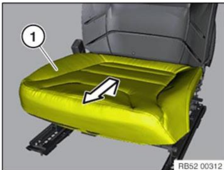
Fig. 60: Removing Seat Cover With Padding Courtesy of BMW OF NORTH AMERICA, INC.
