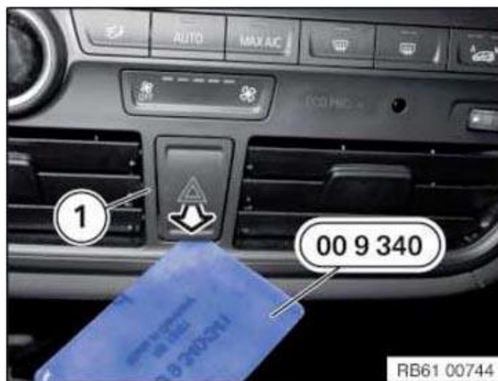
Fig. 613: Removing Hazard Warning Lights System Switch Using Special Tool (00 9 340)
