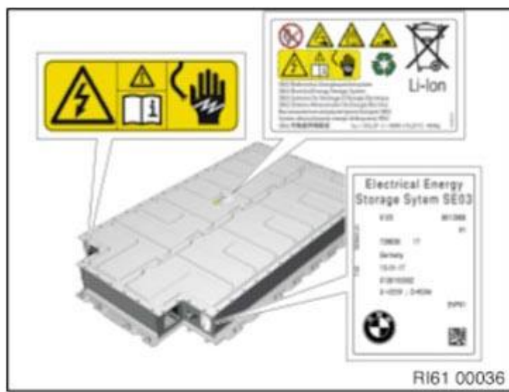
Fig. 291: Identifying High-Voltage Battery Unit Test Device Information Label Courtesy of BMW OF NORTH AMERICA, INC.
