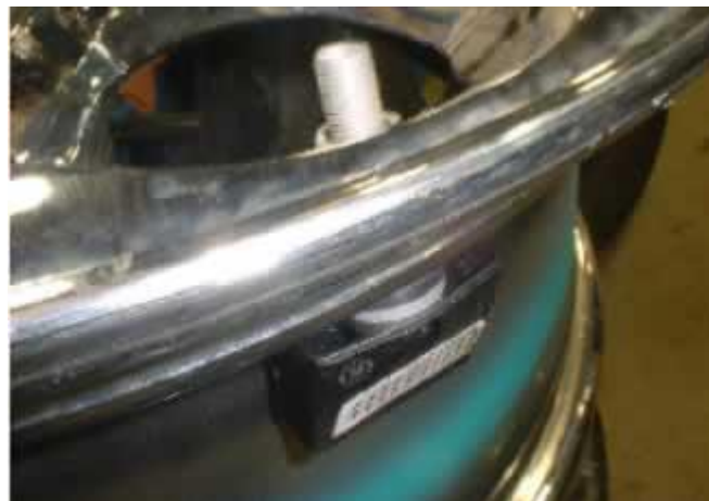
Fig. 16: Valve Stem Mounted Sensor
