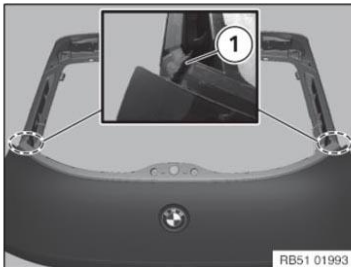
Fig. 229: Identifying Adhesive Bead Applying Area On Tailgate Courtesy of BMW OF NORTH AMERICA, INC.
