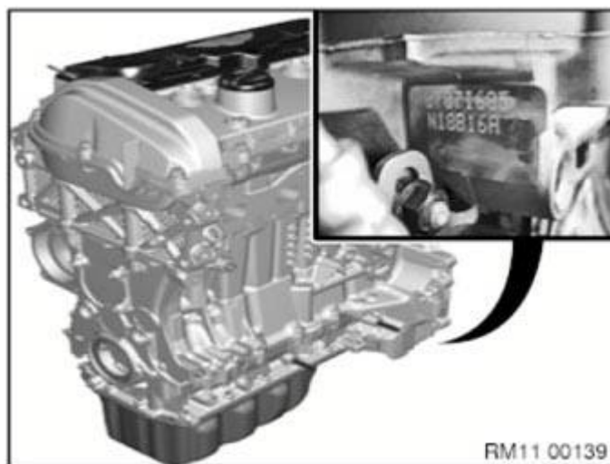
Fig. 28: Identifying Engine Identification Mark - W16 Courtesy of BMW OF NORTH AMERICA, INC.
