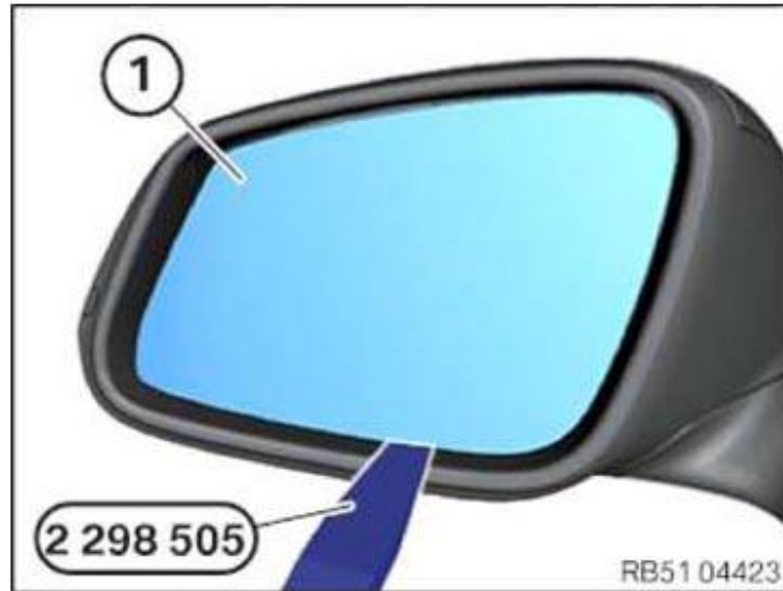
Fig. 135: Unclipping Mirror Glass With Special Tool (2 298 505) Courtesy of BMW OF NORTH AMERICA, INC.
