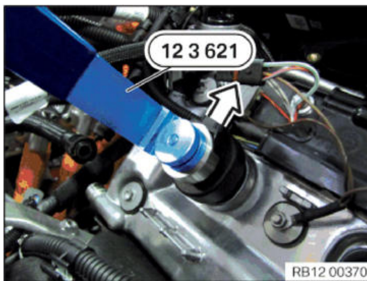
Fig. 37: Pushing Special Tool (12 3 621) Onto Ignition Coil Courtesy of BMW OF NORTH AMERICA, INC.
