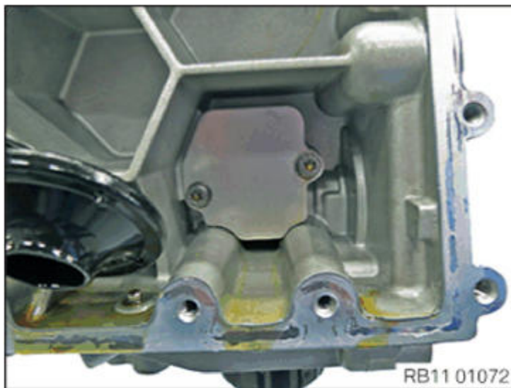
Fig. 276: Identifying Surge Plates On Crankcase Courtesy of BMW OF NORTH AMERICA, INC.
