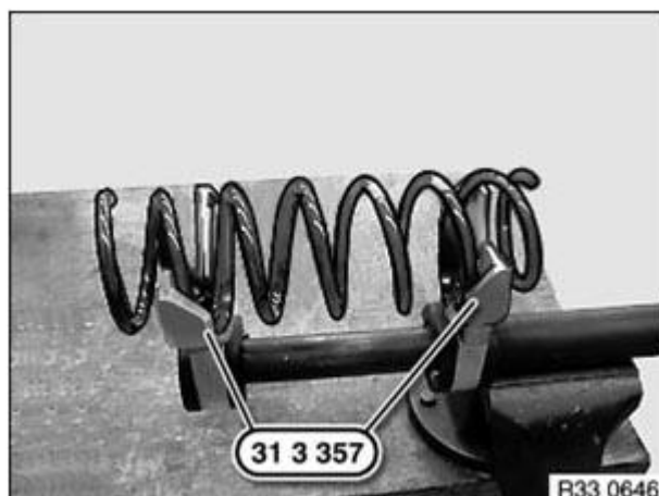
Fig. 85: Identifying Coil Spring And Special Tool (31 3 357)
