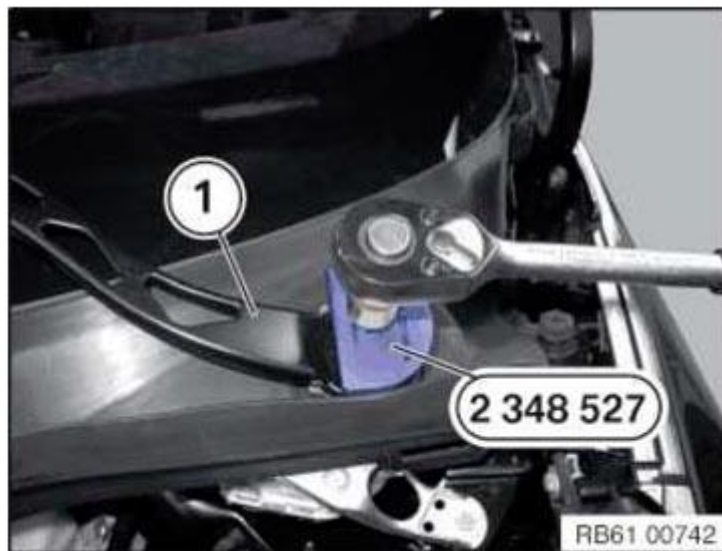
Fig. 681: Pulling Off Wiper Arm Using Special Tool (2 348 527) Courtesy of BMW OF NORTH AMERICA, INC.
