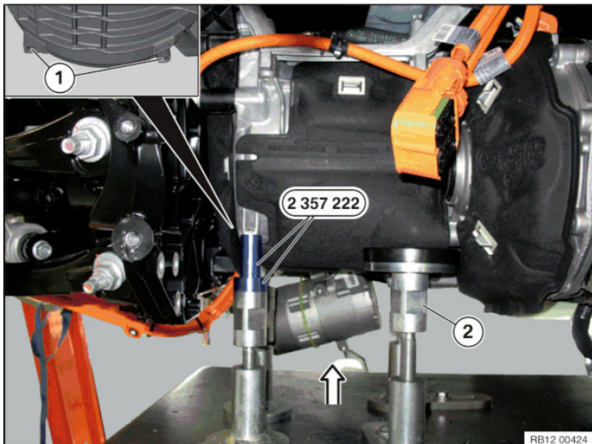
Fig. 154: Positioning Special Tool (2 357 222) At Mounting Points Of Electrical Machine Courtesy of BMW OF NORTH AMERICA, INC.
