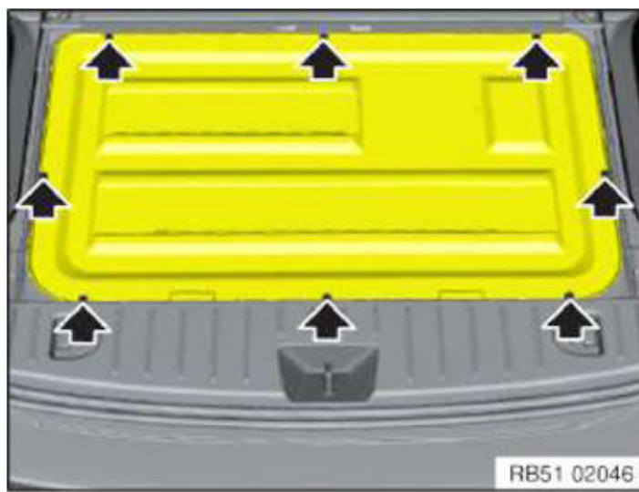
Fig. 387: Locating Luggage Compartment Service Cap Neoprene Nuts Courtesy of BMW OF NORTH AMERICA, INC.
