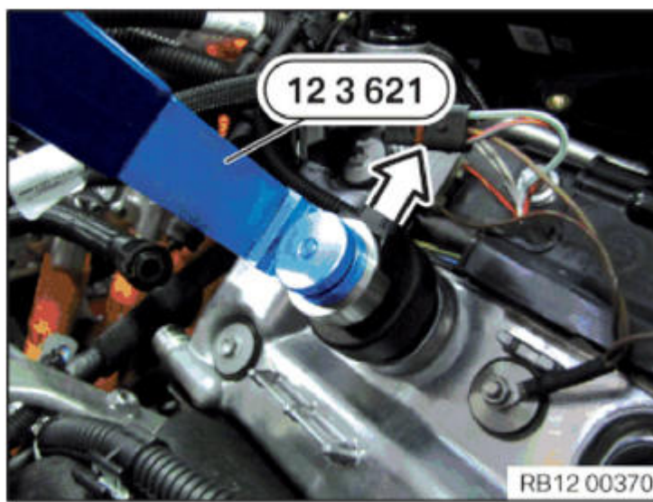
Fig. 2: Pushing Special Tool (12 3 621) Onto Ignition Coil Courtesy of BMW OF NORTH AMERICA, INC.
