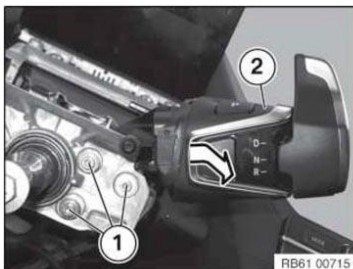
Fig. 603: Removing Gear Selector Switch Courtesy of BMW OF NORTH AMERICA, INC.
