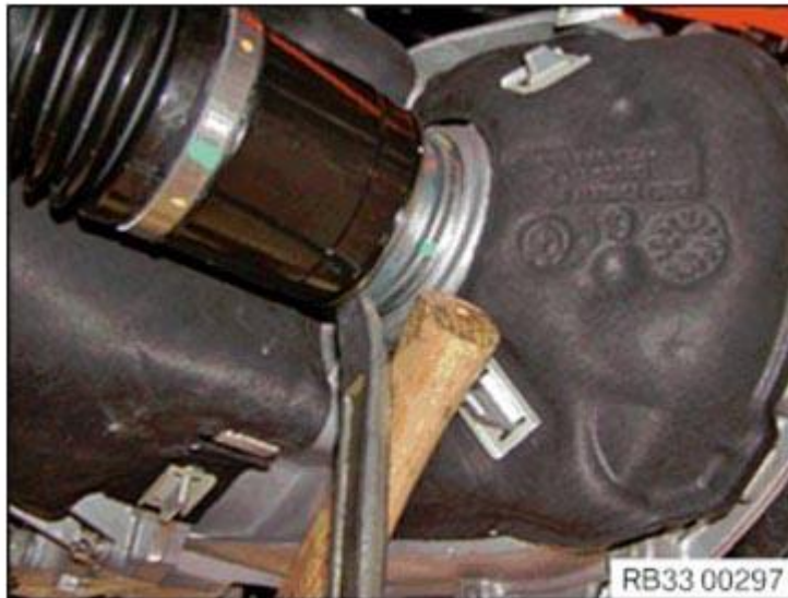
Fig. 12: Supporting Output Shaft Mounting Lever Using Wooden Piece Courtesy of BMW OF NORTH AMERICA, INC.
