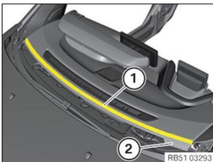
Fig. 249: Identifying Aperture And Foam Tape Courtesy of BMW OF NORTH AMERICA, INC.
