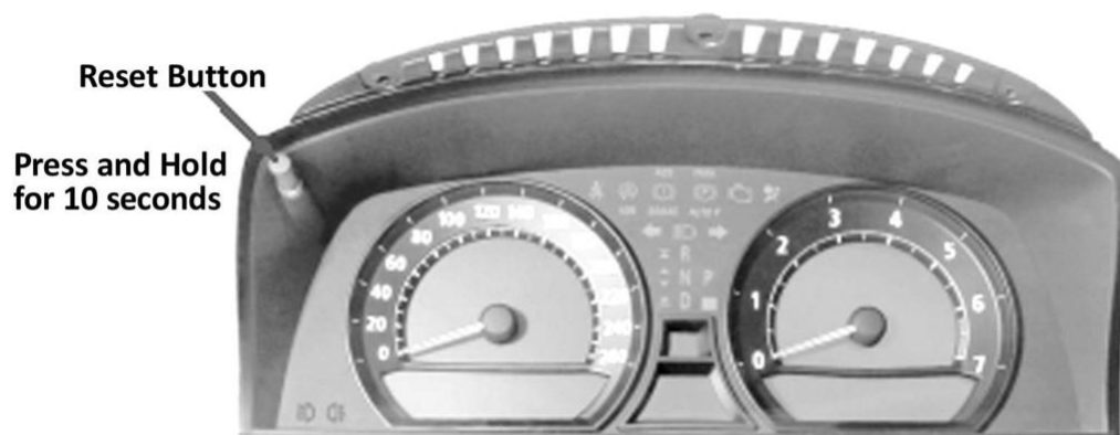
Fig. 8: Identifying Condition Based Service (CBS) Instrument Panel Controls (Typical) Courtesy of BMW OF NORTH AMERICA, INC.
