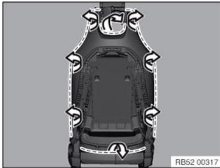
Fig. 52: Lifting Out Welt From Backrest Frame Courtesy of BMW OF NORTH AMERICA, INC.
