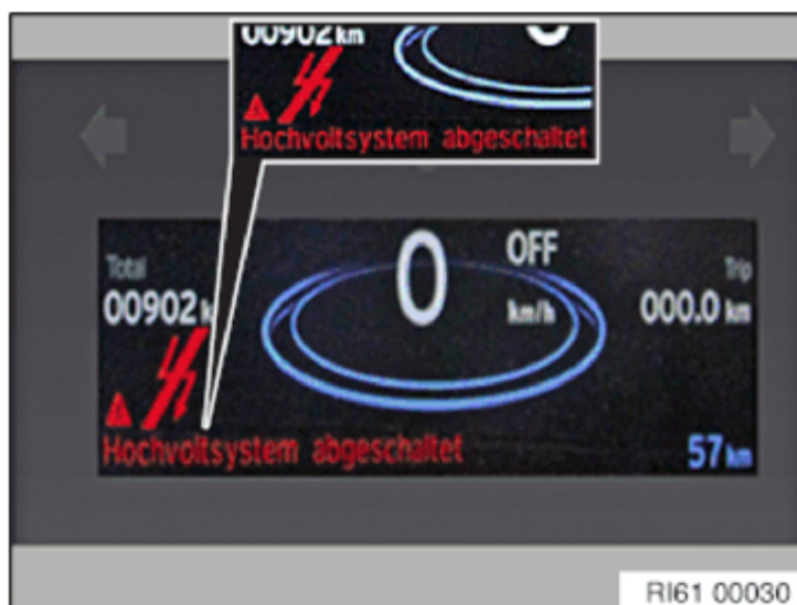
Fig. 166: Screen Display - Check Control Message High-Voltage System Deactivated
