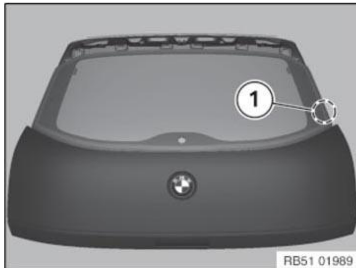
Fig. 225: Identifying String Out Of Spider Sliding Area Through Adhesive Bead Courtesy of BMW OF NORTH AMERICA, INC.
