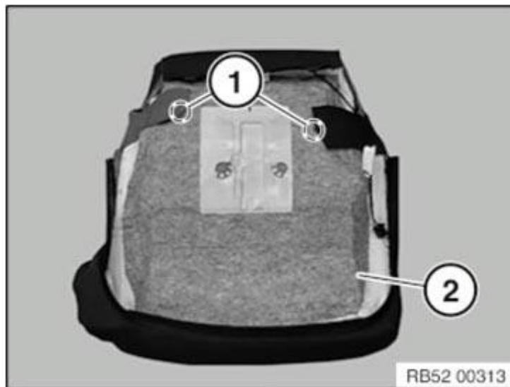
Fig. 71: Identifying Seat Cover And Clamps Courtesy of BMW OF NORTH AMERICA, INC.
