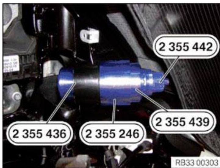
Fig. 64: Pulling Rubber Mount Using Special Tools Courtesy of BMW OF NORTH AMERICA, INC.
