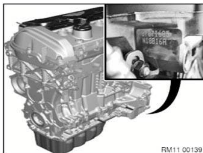
Fig. 25: Identifying Engine Identification Mark - W16 Courtesy of BMW OF NORTH AMERICA, INC.
