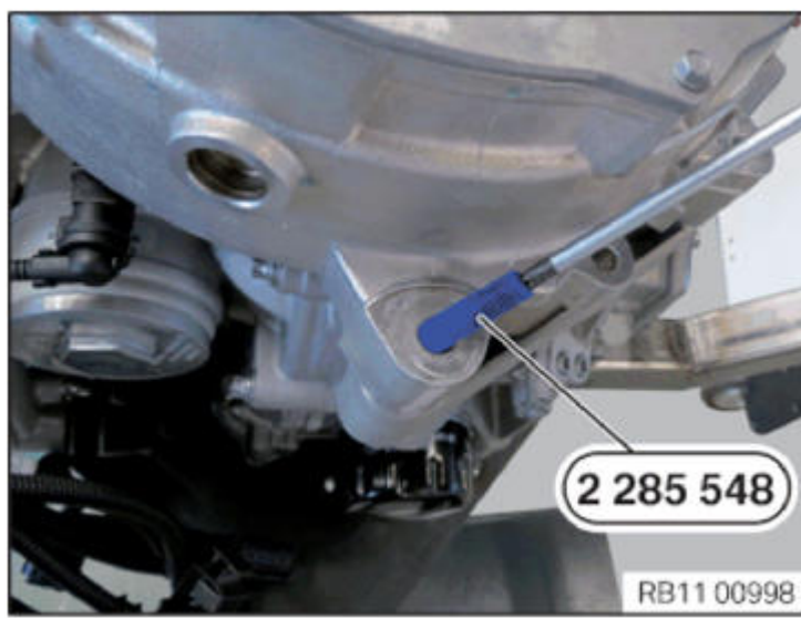
Fig. 109: Screwing Special Tool (2 285 548) Into Bolting Points Courtesy of BMW OF NORTH AMERICA, INC.
