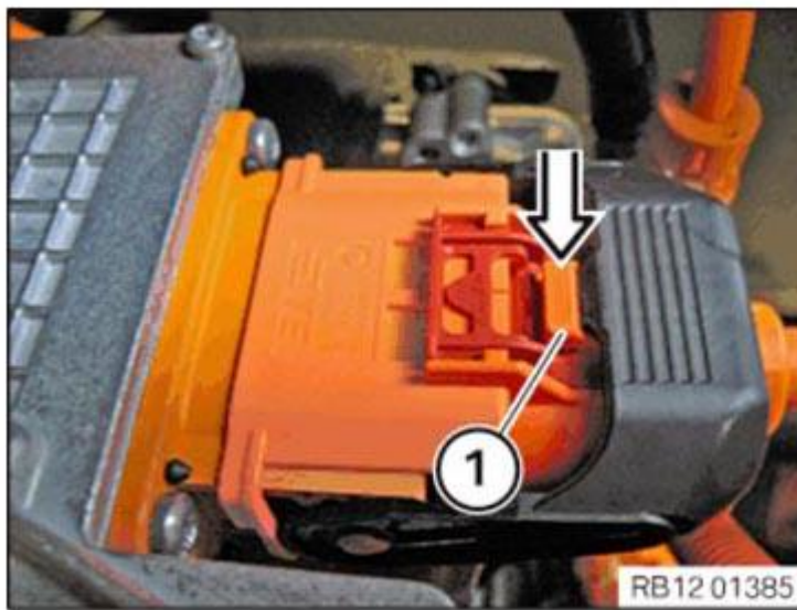
Fig. 26: Pressing High Voltage Connector Lock Courtesy of BMW OF NORTH AMERICA, INC.
