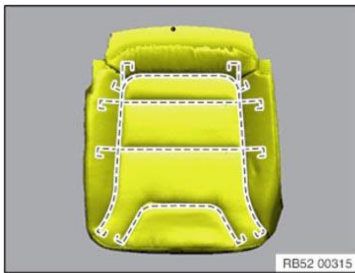
Fig. 63: Identifying Trim Wires Area In Seat Cover Courtesy of BMW OF NORTH AMERICA, INC.
