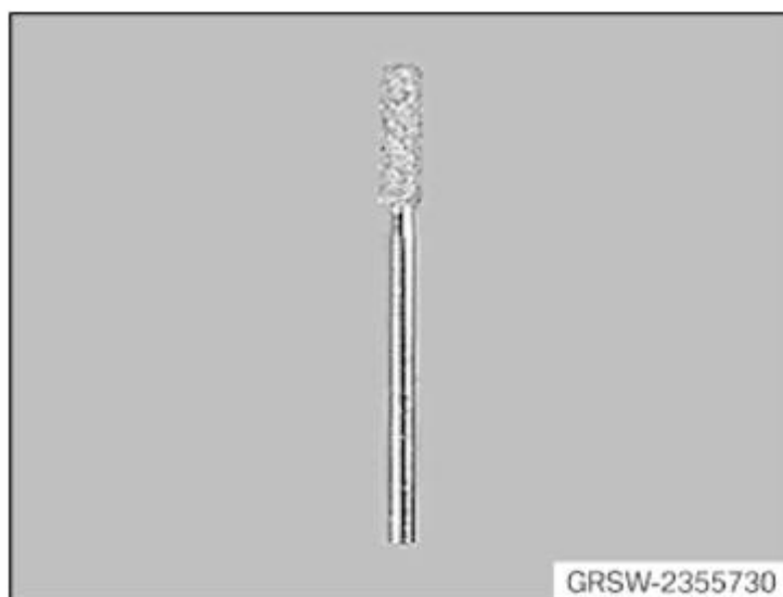
Fig. 16: Identifying Milling Cutter Minimum Set (2355730) Courtesy of BMW OF NORTH AMERICA, INC.
