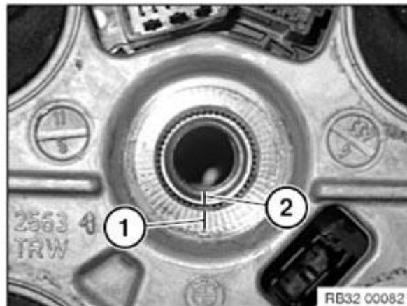
Fig. 53: Identifying Steering Wheel And Steering Column Marking Courtesy of BMW OF NORTH AMERICA, INC.
