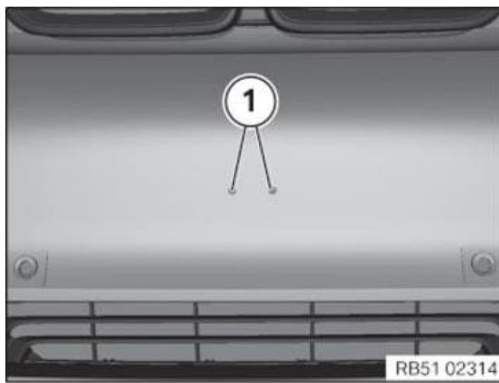
Fig. 18: Identifying Drilling Marks On Bumper Courtesy of BMW OF NORTH AMERICA, INC.
