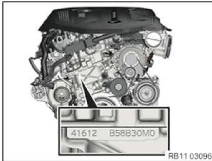
Fig. 32: Identifying Engine Identification Mark - B58 Courtesy of BMW OF NORTH AMERICA, INC.
