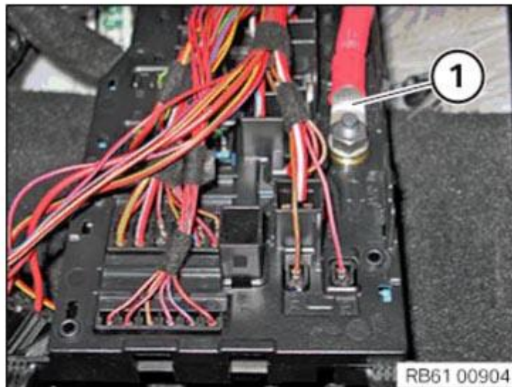
Fig. 269: Identifying Positive Battery Cable Nut Courtesy of BMW OF NORTH AMERICA, INC.
