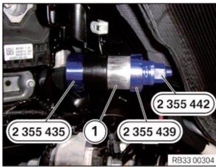
Fig. 49: Installing Rubber Mount Using Special Tools Courtesy of BMW OF NORTH AMERICA, INC.
