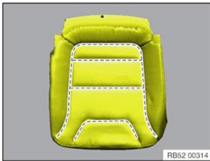
Fig. 72: Identifying Trim Wires Clamps Area Courtesy of BMW OF NORTH AMERICA, INC.
