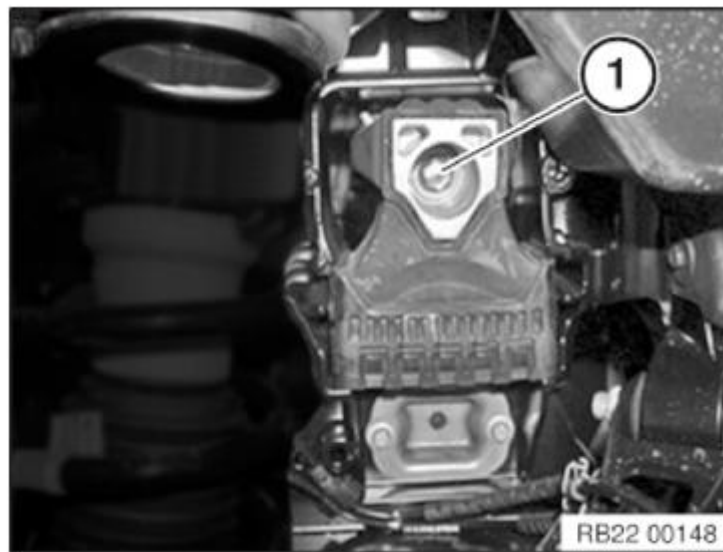
Fig. 6: Identifying Range Extender Transmission Mounting Bracket Screw Courtesy of BMW OF NORTH AMERICA, INC.
