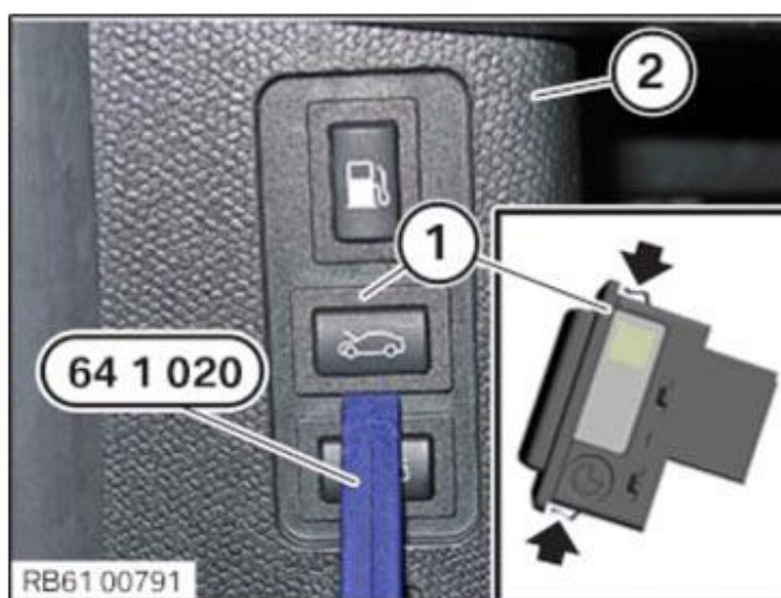
Fig. 77: Removing Engine Compartment Unlocking Switch From Trim Panel Using Special Tool (64 1 020)
