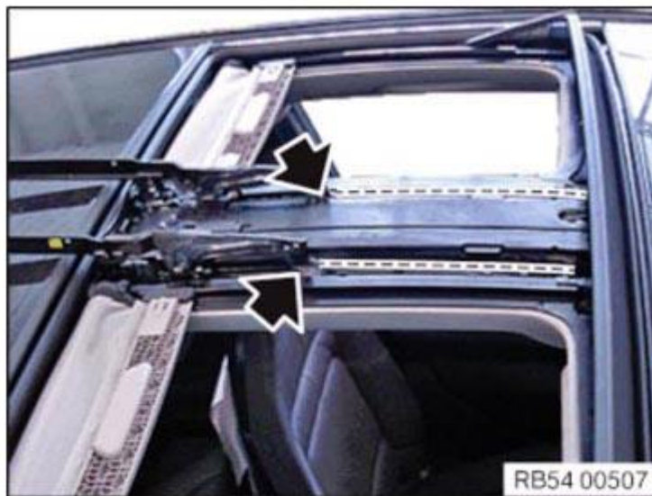
Fig. 5: Locating Slider And Guide Rail Courtesy of BMW OF NORTH AMERICA, INC.
