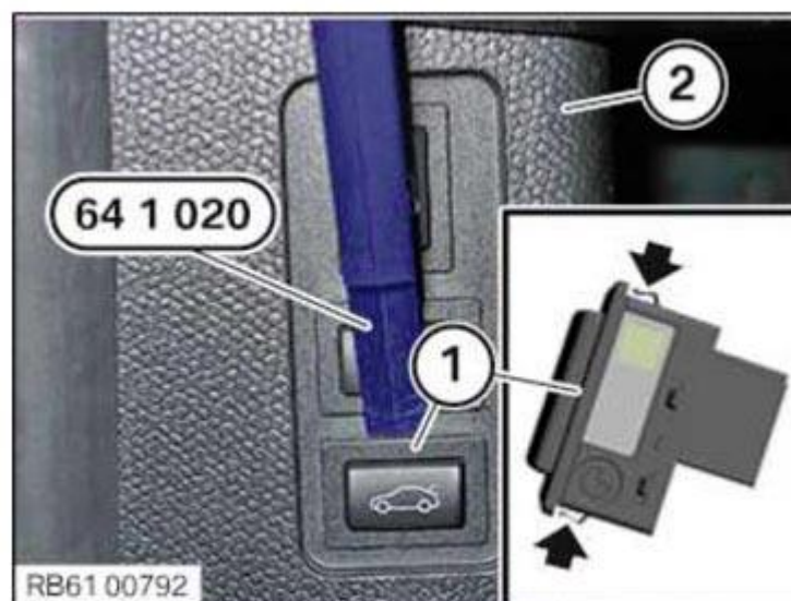
Fig. 592: Removing Tailgate Release Switch From Trim Panel Using Special Tool (64 1 020) Courtesy of BMW OF NORTH AMERICA, INC.
