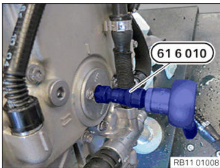
Fig. 249: Releasing Screw Plug With Special Tool (61 6 010) Courtesy of BMW OF NORTH AMERICA, INC.
