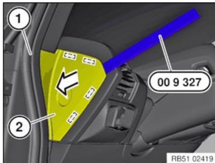
Fig. 364: Removing Side Panel From Dashboard With Special Tool (00 9 327)
