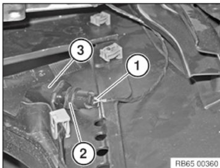
Fig. 59: Identifying Outside Temperature Sensor, Plug Connection And Fixture Courtesy of BMW OF NORTH AMERICA, INC.
