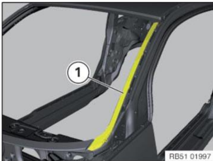
Fig. 248: Identifying Plastic Adhesive Applying Area On Side Frame And A-Pillar Courtesy of BMW OF NORTH AMERICA, INC.
