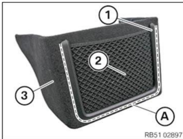
Fig. 372: Identifying Trim Panel, Frame And Storage Net Courtesy of BMW OF NORTH AMERICA, INC.
