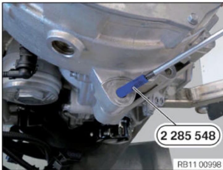
Fig. 140: Screwing Special Tool (2 285 548) Into Bolting Points Courtesy of BMW OF NORTH AMERICA, INC.
