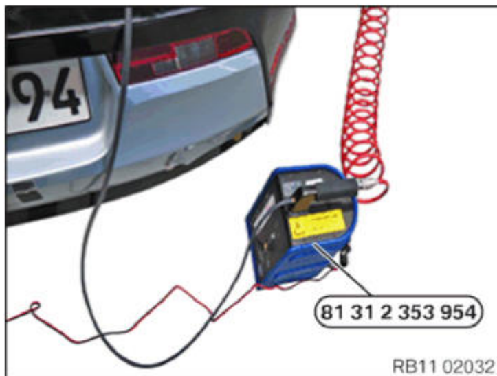
Fig. 83: Preparing Special Tool (81 31 2 353 954) Courtesy of BMW OF NORTH AMERICA, INC.
