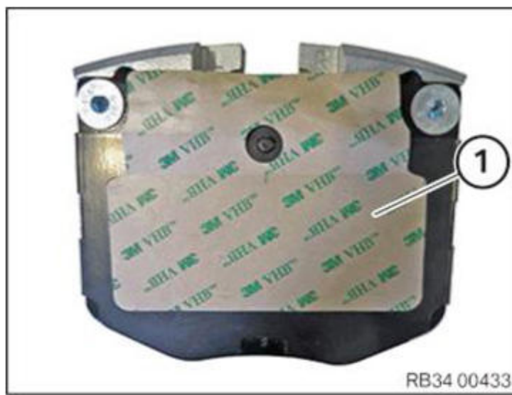
Fig. 61: Identifying Brake Pads Adhesive Layer Courtesy of BMW OF NORTH AMERICA, INC.
