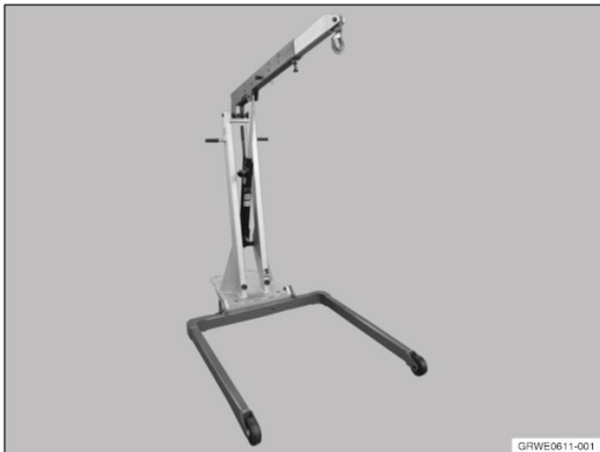
Fig. 93: Identifying Workshop Crane (2220718) Courtesy of BMW OF NORTH AMERICA, INC.
