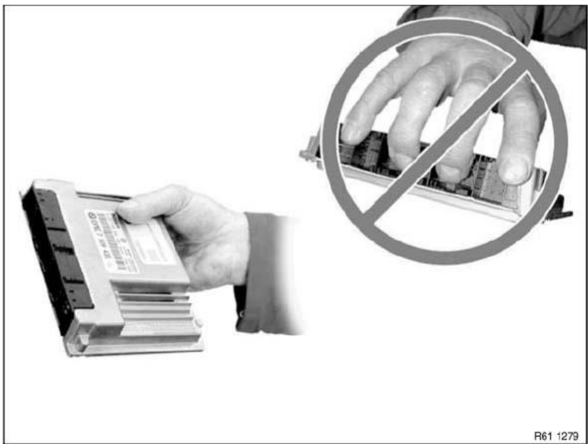
Fig. 639: Caution - Do Not Touch Pins And Multi-Pin Connectors Directly Courtesy of BMW OF NORTH AMERICA, INC.
