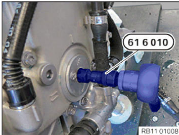
Fig. 187: Releasing Screw Plug With Special Tool (61 6 010). Courtesy of BMW OF NORTH AMERICA, INC.
