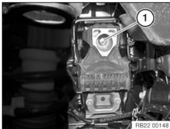
Fig. 1: Identifying Range Extender Transmission Mounting Bracket Screw Courtesy of BMW OF NORTH AMERICA, INC.
