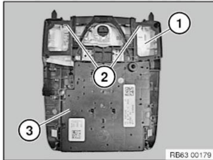
Fig. 626: Identifying Interior Roof Light, Clamps And Roof Switch Cluster Courtesy of BMW OF NORTH AMERICA, INC.
