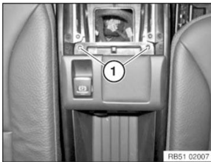
Fig. 90: Identifying Center Console Decorative Trim Screws Courtesy of BMW OF NORTH AMERICA, INC.
