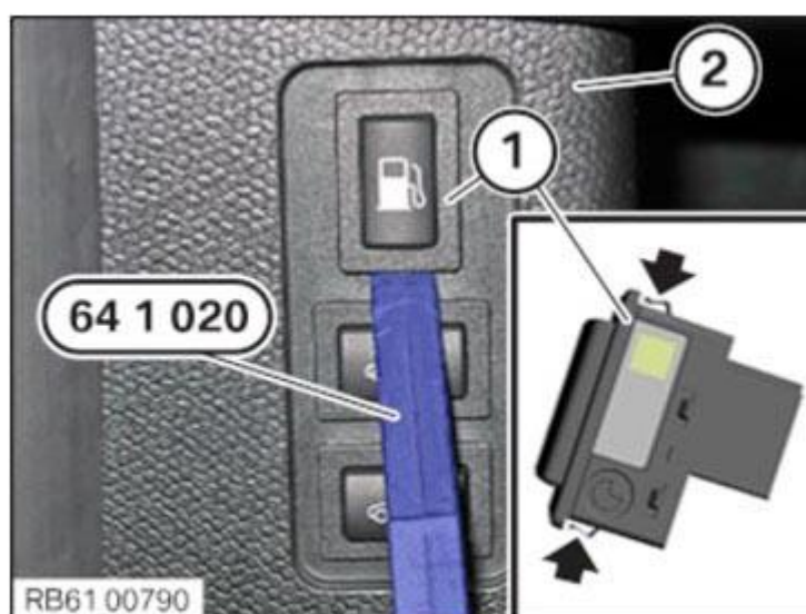
Fig. 588: Prying Fuel Filler Door Release Switch Out Of Trim Panel Courtesy of BMW OF NORTH AMERICA, INC.
