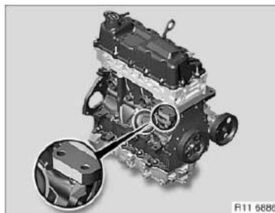
Fig. 24: Identifying Engine Identification Mark - W10/W11 Courtesy of BMW OF NORTH AMERICA, INC.
