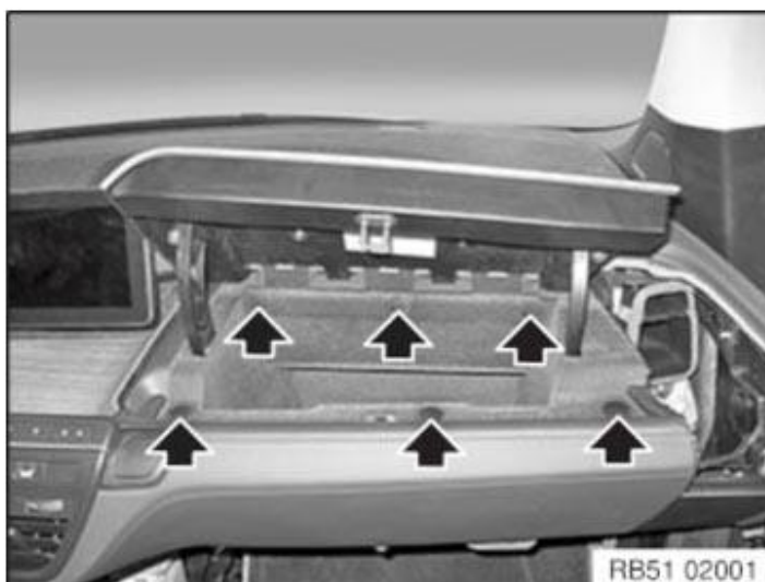
Fig. 126: Locating Glove Box Cover Protective Caps Courtesy of BMW OF NORTH AMERICA, INC.
