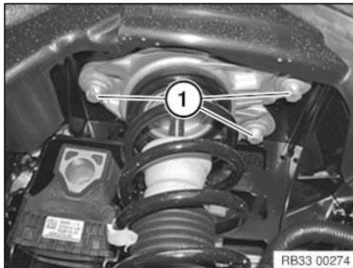
Fig. 79: Identifying Spring Strut Support Bearing Screws Courtesy of BMW OF NORTH AMERICA, INC.
