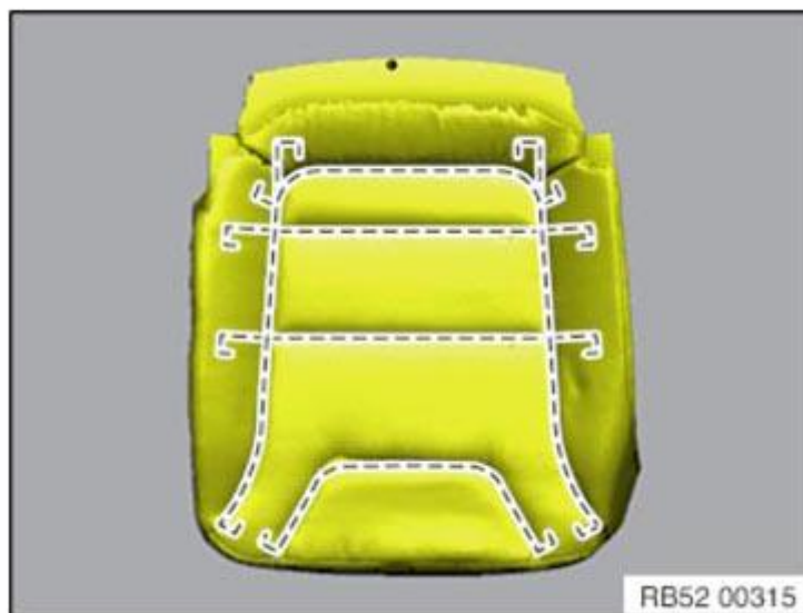
Fig. 73: Identifying Trim Wires Area In Seat Cover Courtesy of BMW OF NORTH AMERICA, INC.
