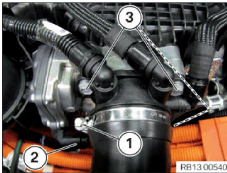
Fig. 8: Identifying Throttle Body Clamp, Connector And Screws Courtesy of BMW OF NORTH AMERICA, INC.
