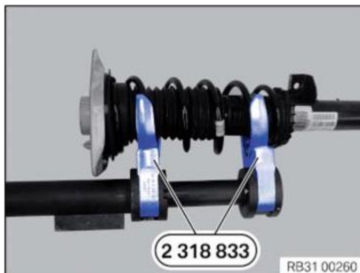
Fig. 58: Accommodating Coil Spring Using Special Tools (2 318 833) Courtesy of BMW OF NORTH AMERICA, INC.
