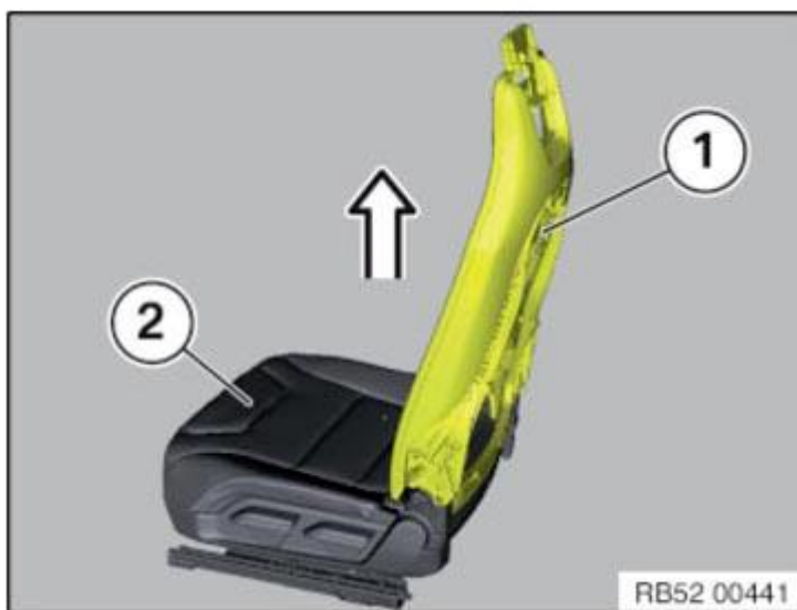
Fig. 16: Removing Backrest Frame From Seat Mechanism
