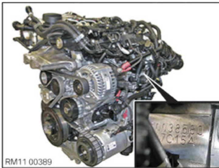
Fig. 29: Identifying Engine Identification Mark - B37/B38A/B47/B48A Courtesy of BMW OF NORTH AMERICA, INC.
