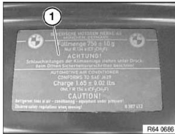
Fig. 103: Identifying Refrigerant Capacity Type Plate Courtesy of BMW OF NORTH AMERICA, INC.
