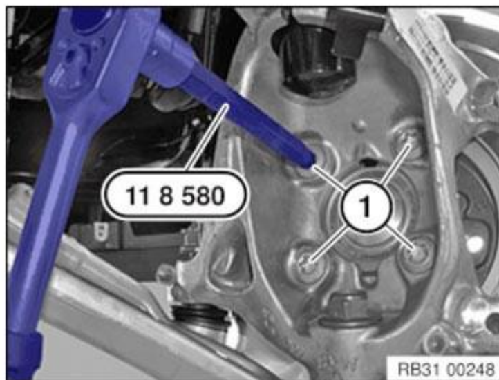
Fig. 55: Removing Front Wheel Bearing Screws Using Special Tool (11 8 580) Courtesy of BMW OF NORTH AMERICA, INC.
