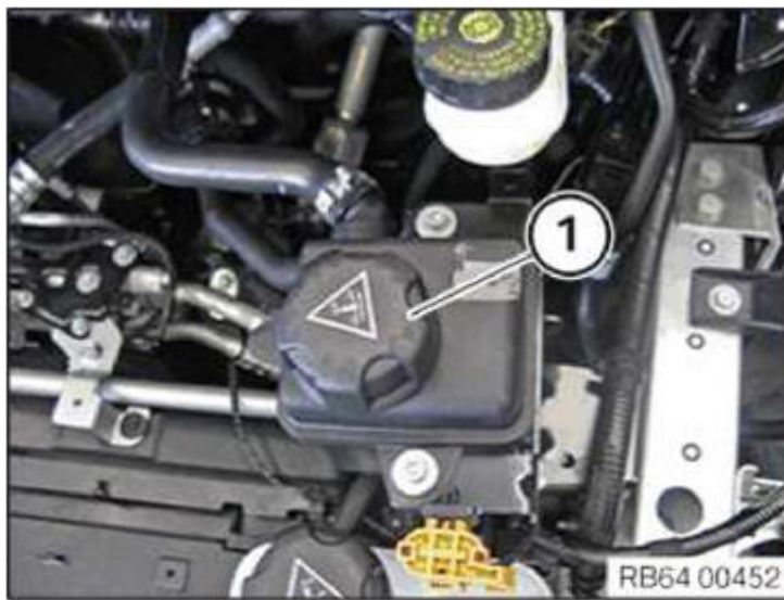
Fig. 3: Identifying Sealing Cap On Coolant Expansion Tank Courtesy of BMW OF NORTH AMERICA, INC.
