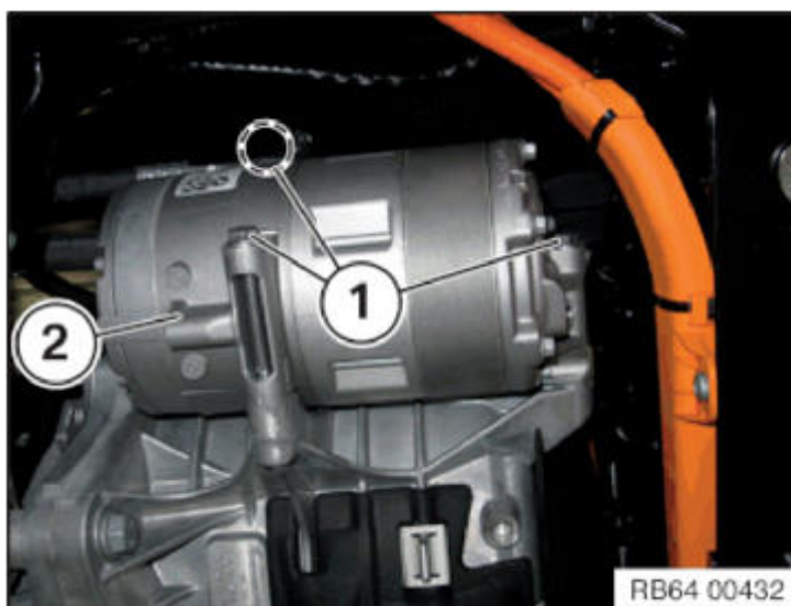
Fig. 340: Identifying Air Conditioning Compressor And Screw Courtesy of BMW OF NORTH AMERICA, INC.
