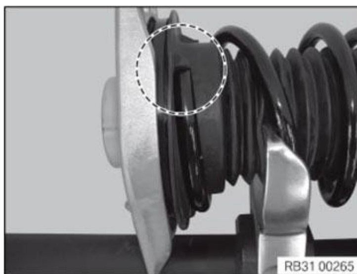
Fig. 61: Checking Top Spring Pad Position Courtesy of BMW OF NORTH AMERICA, INC.
