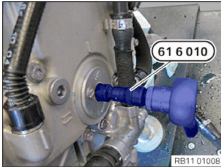
Fig. 215: Releasing Screw Plug With Special Tool (61 6 010). Courtesy of BMW OF NORTH AMERICA, INC.
