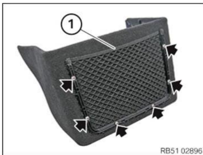
Fig. 370: Identifying Storage Net With Screws Courtesy of BMW OF NORTH AMERICA, INC.
