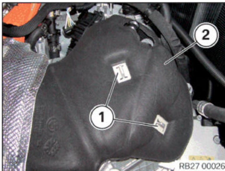
Fig. 51: Identifying Sound Insulation And Clamps Courtesy of BMW OF NORTH AMERICA, INC.
