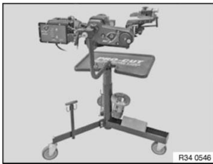
Fig. 66: Identifying Mobile Brake Disc Lathe Courtesy of BMW OF NORTH AMERICA, INC.
