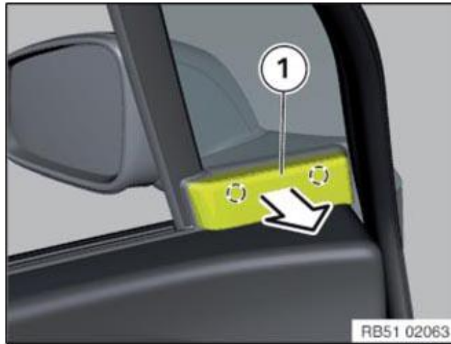
Fig. 150: Removing Window Frame Cover Courtesy of BMW OF NORTH AMERICA, INC.
