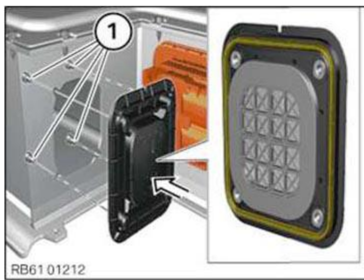
Fig. 323: Installing Venting Unit Courtesy of BMW OF NORTH AMERICA, INC.
