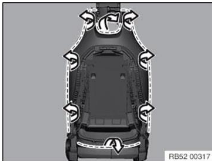
Fig. 45: Lifting Out Welt From Backrest Frame Courtesy of BMW OF NORTH AMERICA, INC.
