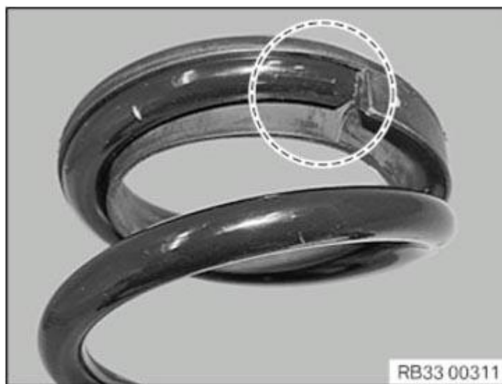
Fig. 90: Checking Top Spring Pad Positioning Courtesy of BMW OF NORTH AMERICA, INC.
