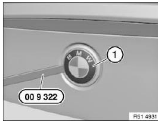
Fig. 70: Removing BMW Badge Using Special Tool (00 9 322) Courtesy of BMW OF NORTH AMERICA, INC.
