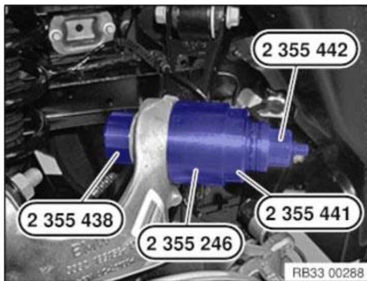
Fig. 70: Pulling Rubber Mount Using Special Tools Courtesy of BMW OF NORTH AMERICA, INC.
