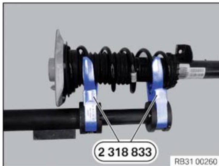
Fig. 83: Accommodating Coil Spring Using Special Tools (2 318 833) Courtesy of BMW OF NORTH AMERICA, INC.
