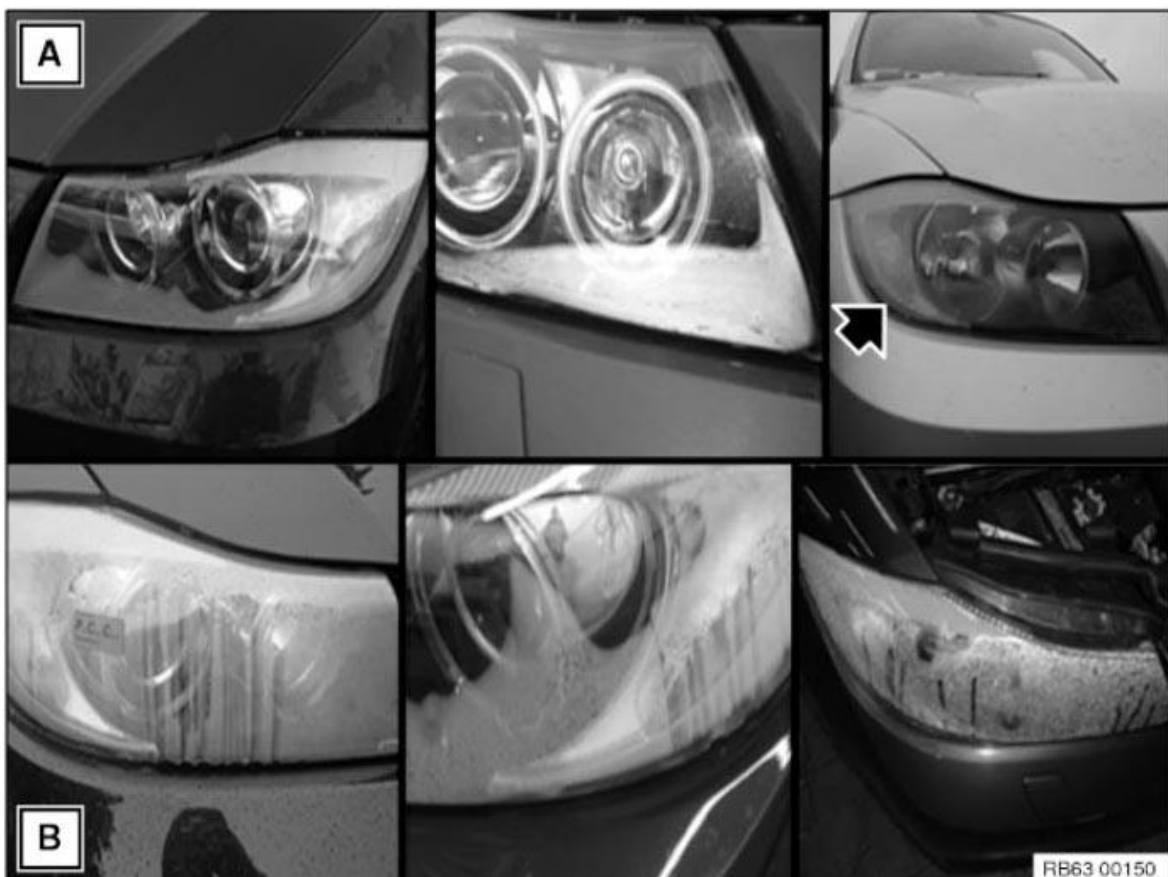
Fig. 32: Identifying Headlight Fogging Fault Pattern Courtesy of BMW OF NORTH AMERICA, INC.
