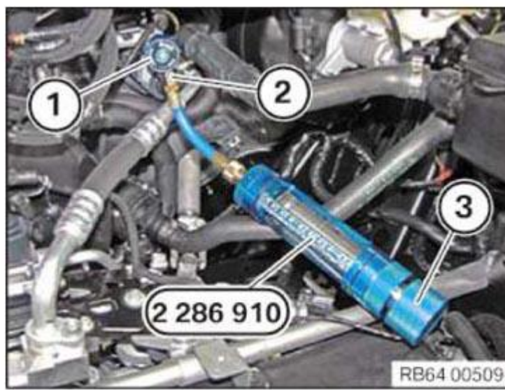
Fig. 105: Identifying Low Pressure Quick-Release Coupling And Screw Courtesy of BMW OF NORTH AMERICA, INC.
