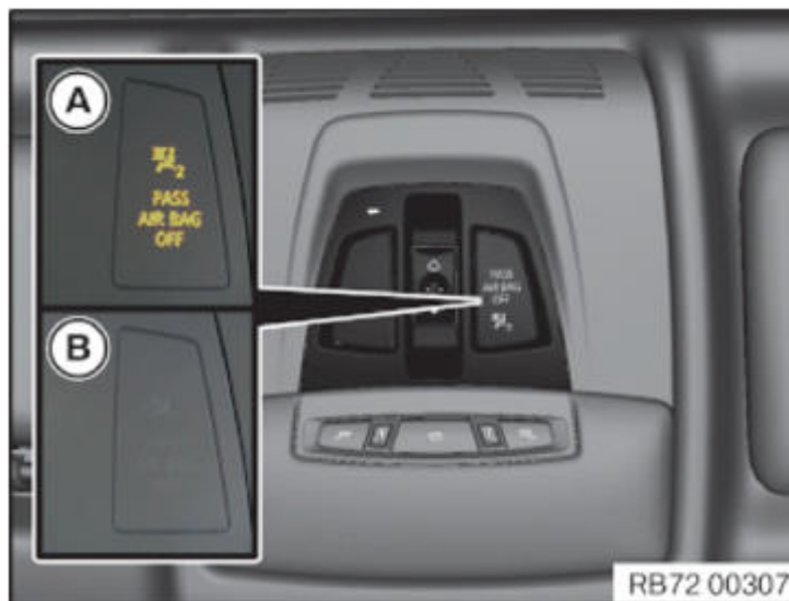
Fig. 18: Identifying Front Passenger Airbags Indicator Light Courtesy of BMW OF NORTH AMERICA, INC.
