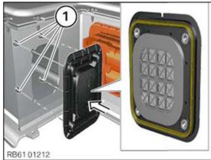
Fig. 453: Installing Venting Unit Courtesy of BMW OF NORTH AMERICA, INC.
