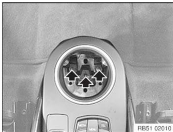
Fig. 73: Locating Center Console Trim Screws Courtesy of BMW OF NORTH AMERICA, INC.
