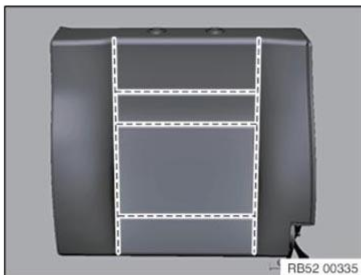
Fig. 90: Identifying Trim Wires And Clamps Area (Marked Area)
