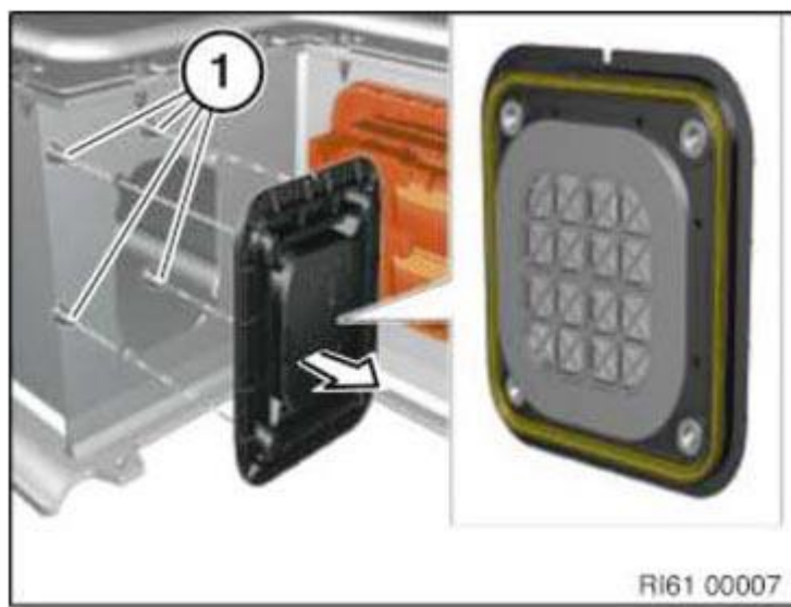
Fig. 491: Removing Degassing Unit Courtesy of BMW OF NORTH AMERICA, INC.
