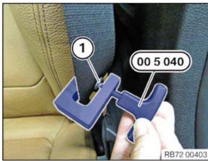
Fig. 2: Pressing Seat Belt Clip With Special Tool (00 5 040). Courtesy of BMW OF NORTH AMERICA, INC.
