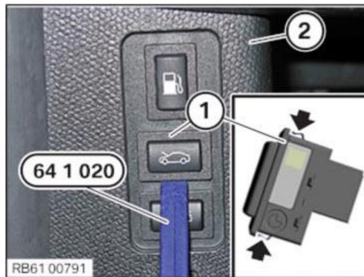
Fig. 586: Removing Engine Compartment Unlocking Switch From Trim Panel Using Special Tool (64 1 020)
