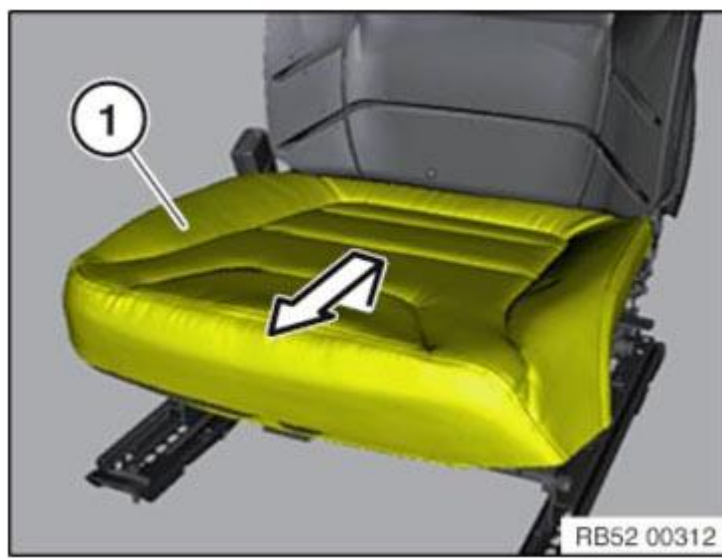
Fig. 70: Removing Seat Cover With Padding Courtesy of BMW OF NORTH AMERICA, INC.
