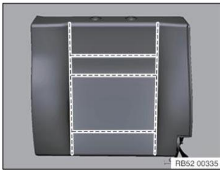
Fig. 95: Identifying Trim Wires And Clamps Area (Marked Area) Courtesy of BMW OF NORTH AMERICA, INC.
