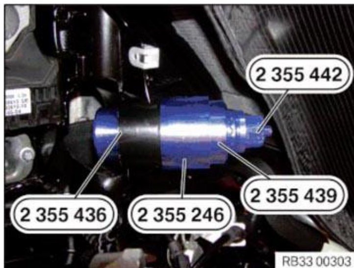
Fig. 48: Removing Rubber Joint Using Special Tools Courtesy of BMW OF NORTH AMERICA, INC.
