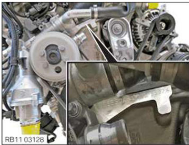
Fig. 23: Identifying Engine Identification Mark - S55 Courtesy of BMW OF NORTH AMERICA, INC.
