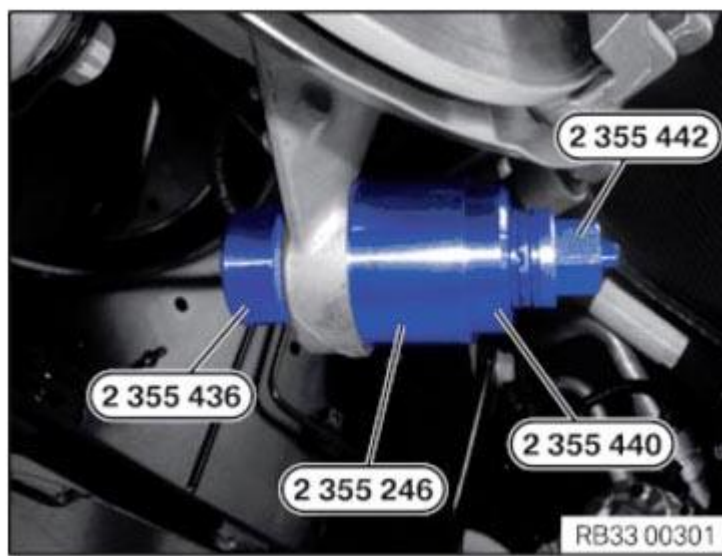
Fig. 67: Removing Rubber Mount Using Special Tools Courtesy of BMW OF NORTH AMERICA, INC.
