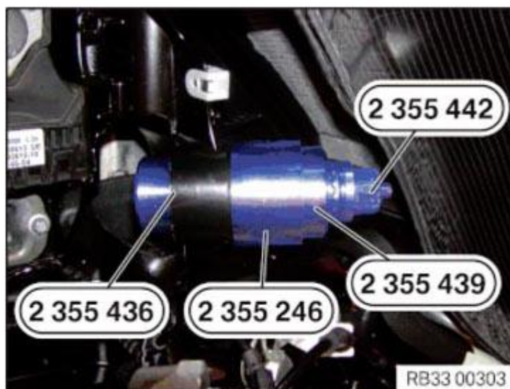
Fig. 68: Pulling Rubber Mount Using Special Tools Courtesy of BMW OF NORTH AMERICA, INC.
