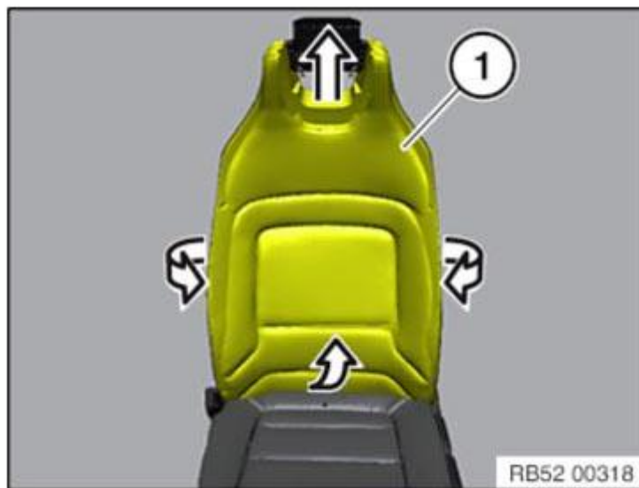
Fig. 53: Pulling Off Backrest Cover With Upholstery From Backrest Frame Courtesy of BMW OF NORTH AMERICA, INC.
