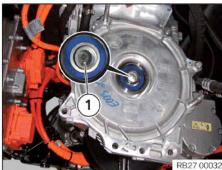
Fig. 69: Identifying Rotor Shaft Courtesy of BMW OF NORTH AMERICA, INC.
