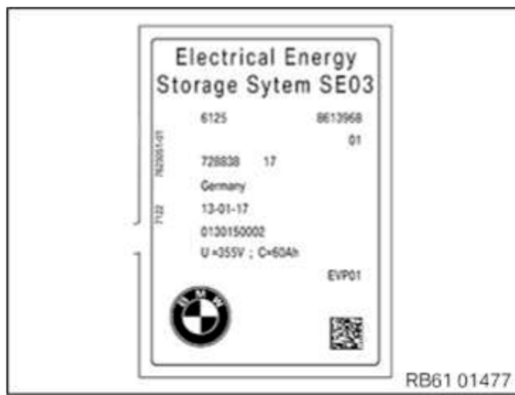
Fig. 450: Identifying Electrical Energy Storage System Type Plate Courtesy of BMW OF NORTH AMERICA, INC.
