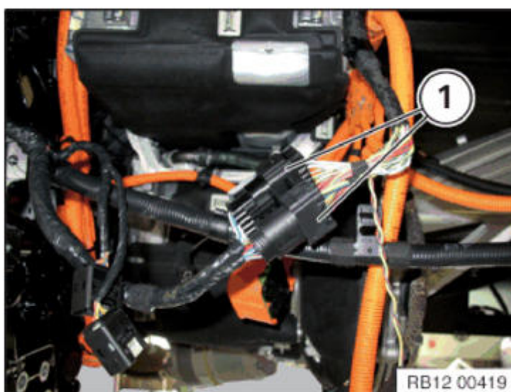
Fig. 163: Identifying Wiring Harness Plug Connections
