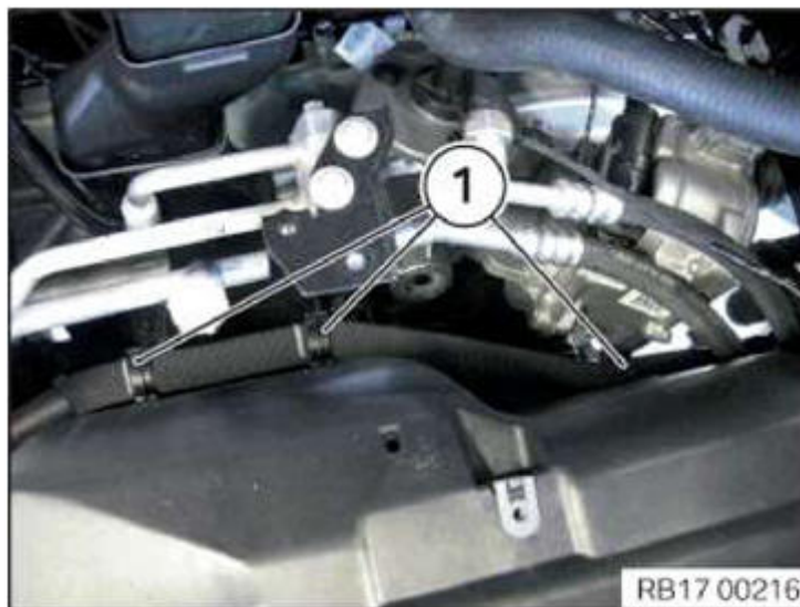
Fig. 75: Identifying Air Duct Coolant Hose Clamps Courtesy of BMW OF NORTH AMERICA, INC.
