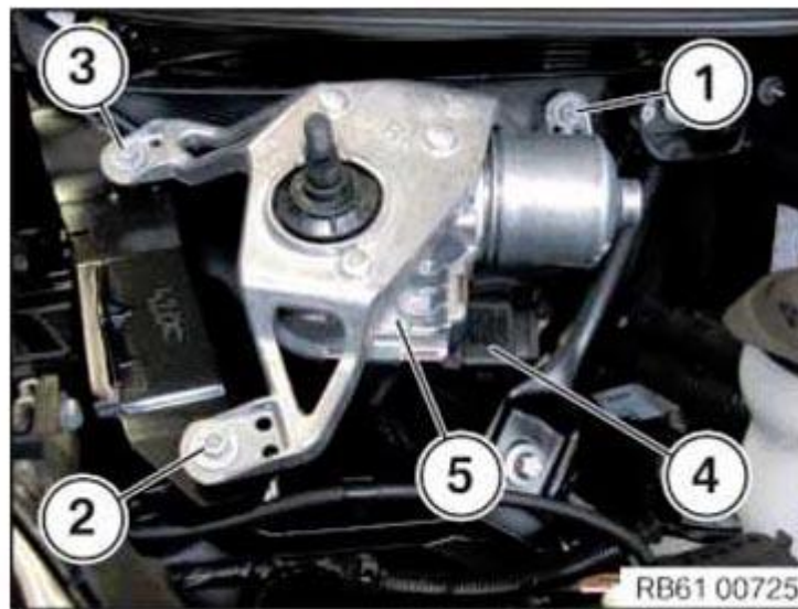
Fig. 672: Identifying Right Wiper Motor, Plug Connection And Nuts Courtesy of BMW OF NORTH AMERICA, INC.
