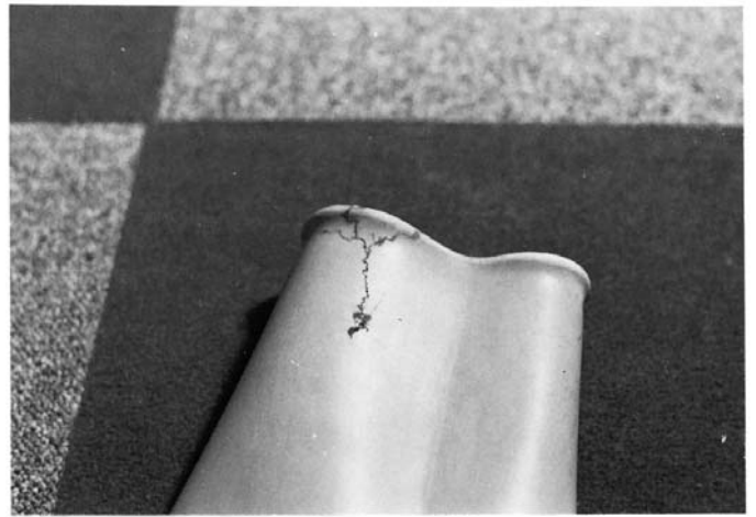
FIG. 25 Tracking—Insufficient Immersion Depth
