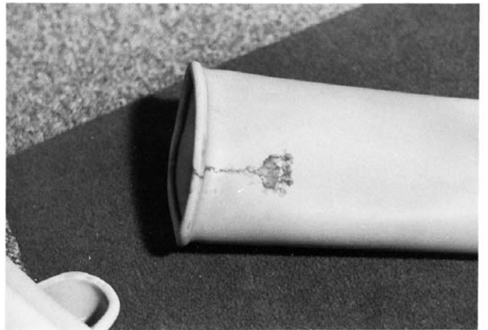
FIG. 26 Tracking—Contaminated Dielectric Fluid
