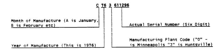
Note: Complete serial number is found only on the Onan nameplate. The six digit actual serial number is stamped on the casting of the engine or generator, sometimes accompanied by a seventh digit denoting factory origin.
