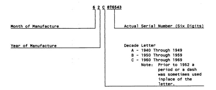
Note: The complete serial number is found only on the Onan nameplate. The six digit actual serial number is stamped on the casting of the engine or generator. Units with missing or damaged nameplate the model can be identified using the serial number microfiche.
