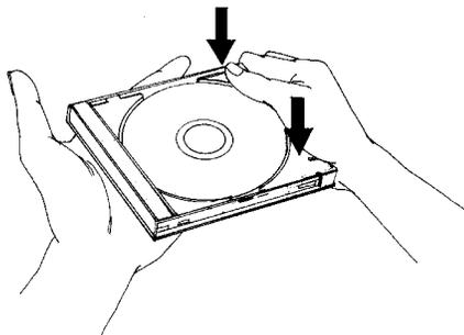
**Caution:** If the caddy appears defective (e.g., warped, cracked, or bent) do not insert it into the drive. A defective caddy can become stuck inside the drive, requiring the drive's return to your dealer for service. If your caddy appears defective, promptly replace it with a new one.
