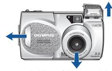
If the lens barrel does not extend, the lens cover is probably not fully open. Slide the lens cover completely to the open position.
