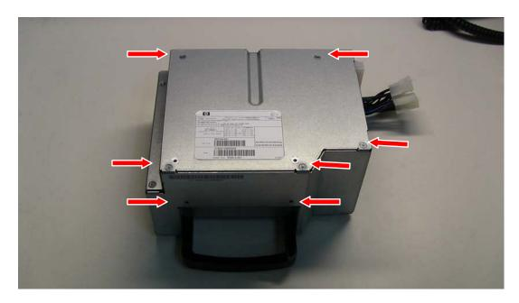
b. Remove all screws from the base of the power supply chassis.
