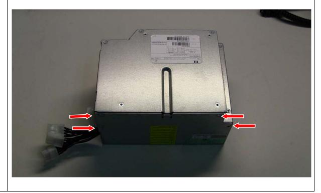
2. Lift and pull handle to remove the top plate of the power supply chassis. The unit will fall open into two parts, as shown in the following figure.
