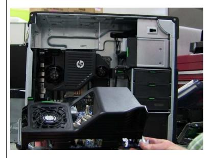
b) Lift riser out of chassis.
