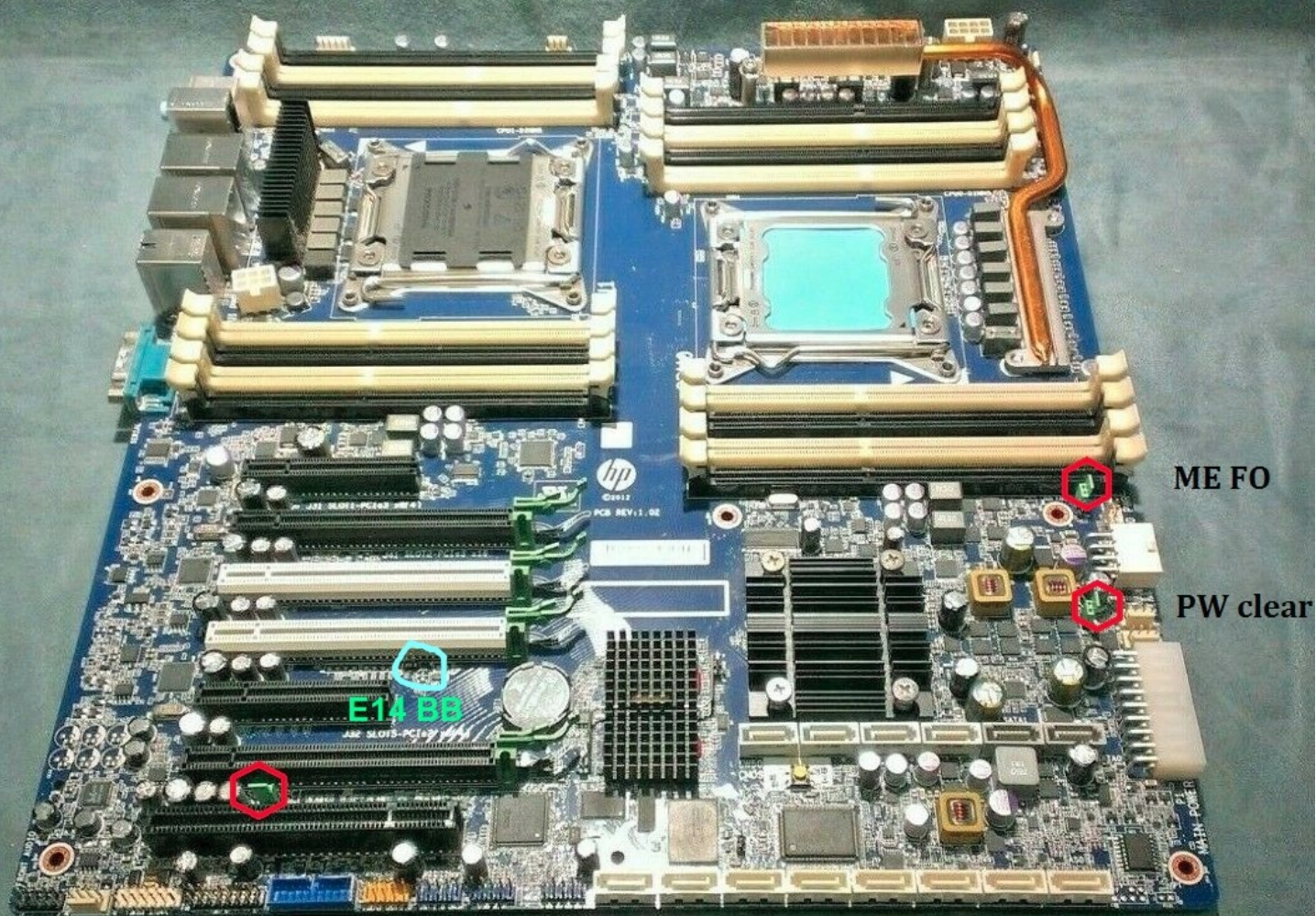
Position of 3 jumpers on later versions of the Z820 motherboards
