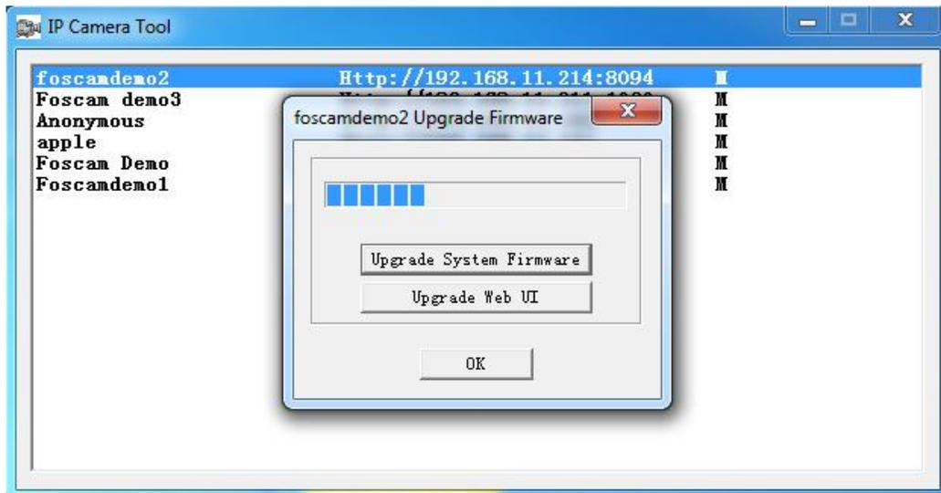
Camera will reboot after upgrading the system firmware. The IP address will disappear from the IP Camera Tool for about 60 seconds. Please upgrade webUI after camera's IP is back to IP Camera Tool.
