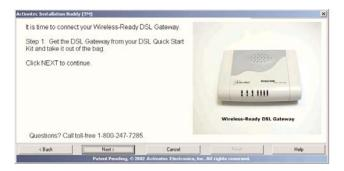
**11.** The next window appears. Plug the smaller end of the **Power Cord** into the **Black Port** on the back of the Gateway, then click **Next**.
