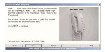
**5.** After the next window appears, plug a **Phone Filter** into ever Phone Jack that has a device (phone, fax machine, answering machine, etc.), then click **Next**.
