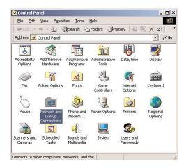
5. In the "Network and Dial-up Connections" window, double-click Local Area Connection. A number may be displayed after the Local Area Connection. If there is more than one Local Area Connection listed, locate the one that corresponds to the network card installed in the computer by finding the name of the network card in the Device Name column.
