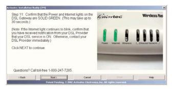
**Note**: If the Power and Internet Lights on the Gateway are not solid green, check all connections to the Gateway. If all connections are plugged in properly, call Qwest DSL Technical Support at 1-800-247-7285.
