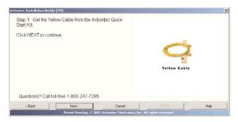
**6.** When the next window appears, plug one end of the **Yellow Ethernet Cable** into one of the **Yellow Ports** on the back of the Gateway, then click **Next**.
