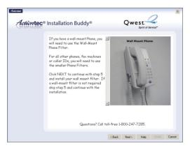
6. Install a wall-mount phone filter by removing the wall-mount telephone and opening the top and bottom toggles. Then, push the wall-mount filter onto the wall jack, push the toggles back into the closed position, and remount the wall-mount telephone. Click Next.
