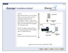
**Caution: Do not** plug a phone filter in the phone jack in which the green DSL cable is plugged.
