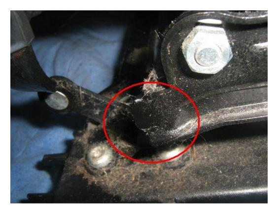
Then flip the seat over and remove the other side and the bolt into the seat belt latch. The plastic cover is held in by a small stud that locates into a hole. Just pull the back of the plastic towards the rear of the car and the stud pops out then you push it forward to detach the slot off the tang on the frame and wiggle it off the seat belt latch holder
