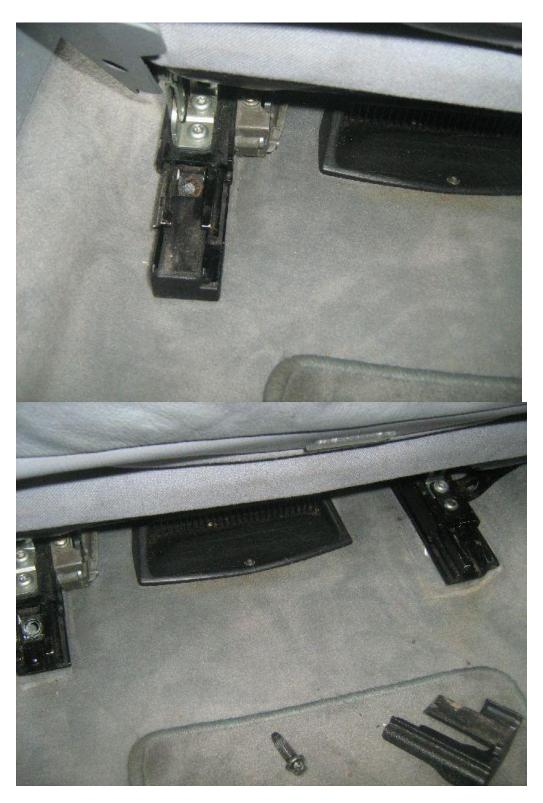
Remove the wiring from the front connectors – the plugs on the door side just pull out but the big connector to the seat module has a slider. As you pull it towards the door it unlatches the connector and pops it out for you.
