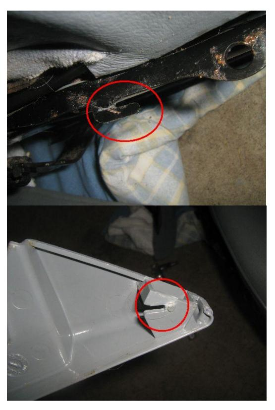
One they are off you can undo the very front bolt and the two rear bolts on each side . this will separate the base and motors from the seat base and the seat back from the seat bottom
