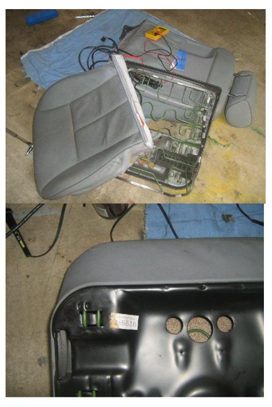
To get to the seat top heater you can remove all of the leather but the most likely place is the left bolster panel so I just removed the back panel and peeled the leather up from the bottom
