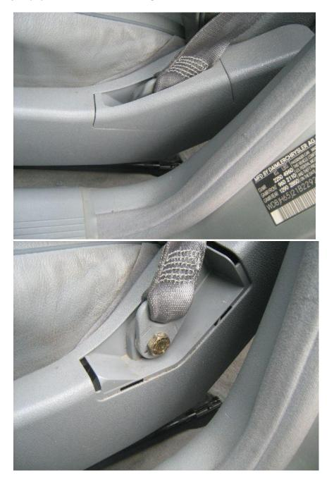
The seat in the right position pull out the rear covers on the seat rails – just finger pressure – to expose the bolts. The fronts are open. It takes a 12mm internal star
