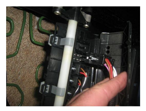
Once you have it out its easy to work on and you now have to separate the back from the bottom. First undo the one screw on the back of the plastic cover that goes from the door side front to back, the rest of the panel pops off once the screw is out and I have marked the connections in red circles. The prong slides into the cover so you actually push the cover towards the front of the car to remove it.
