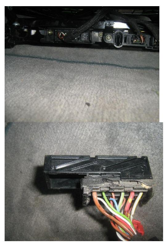
Then just lift out the seat. Make sure you have some blankets or similar on the floor to lay it on, you can also get at nthe wire connectors easier. Undo the 2 bolts and remove the small connector that has the seat heater wires in it.
