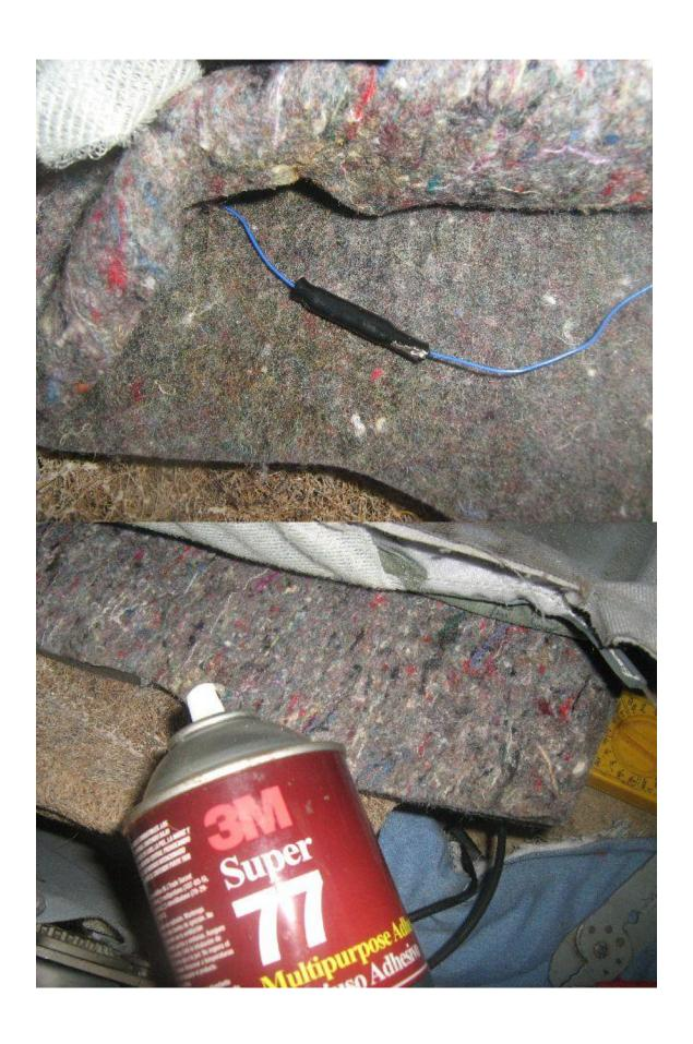
You have to put the crimp and the shrink wrap onto the wire first obviously! Otherwise you are a bit stuck.
