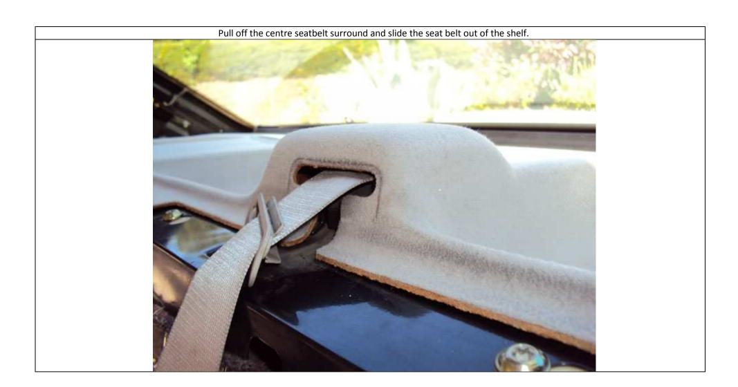
The shelf can now be lifted out. Remember to unclip the rear brake light connector when the shelf is about half way out. Refitting is a reverse of removing.
