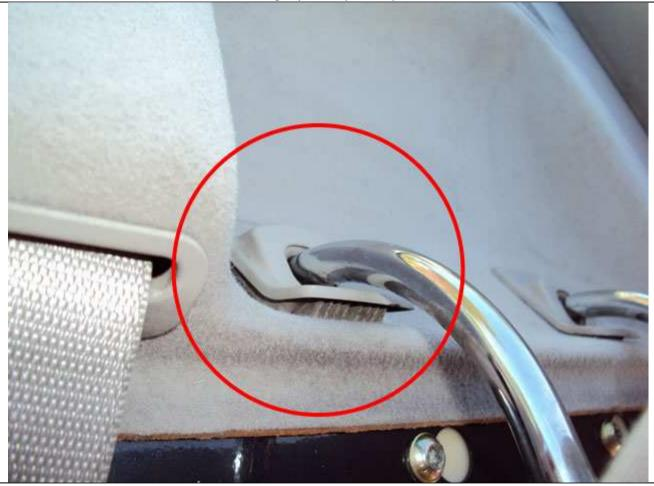
Unclip the black soundproofing (circled) from along the top of the seat just underneath the headrest level and you will see access holes to the headrest mechanism.
