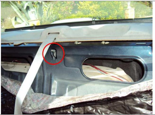
Through the access holes, squeeze the two plastic flaps (a) with your fingers and pop them up through the hole. The surround will now be detached from the shelf. Push the black lever (b) up softly to unlock the headrest arms and slide the arms out of the mechanism a bit at a time until the headrest is removed. Take out all 3 headrests.
