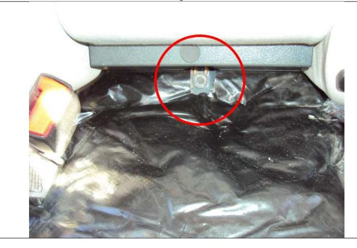
Pull up the rubber door surround and then pop up the side protectors from each side of the seat. Slide the protector down slightly before removing it to unhook the plastic clip at the top (circled).
