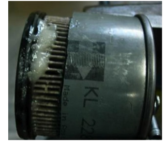
Fuel filter clogging due to (bio) diesel gelling under cold climate conditions
