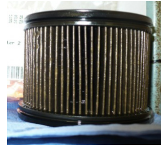
Fuel filter clogging due to soap deposition
