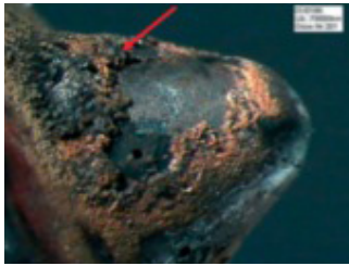
External deposits – fuel injector tip (nozzle coking)
